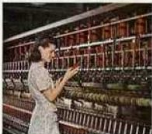
In spinning rooms at a large mill, spools of carded wool, roughly spun and dyed, are twisted and lengthened into a continuous thread.
