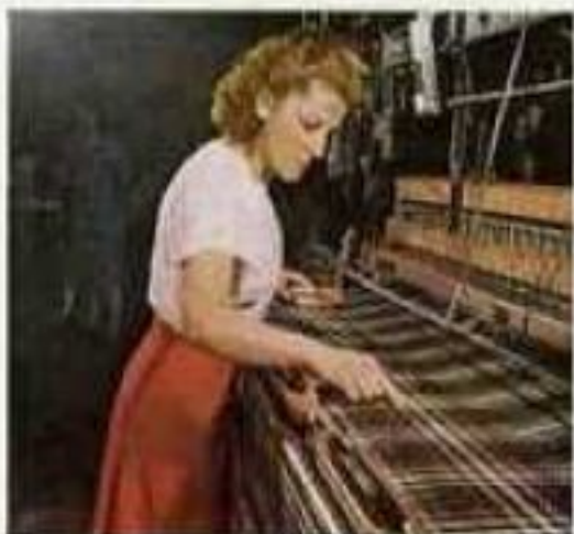
Modern weaving is done on high-speed automatic looms. Bobbin with crosswise threads is shot rapidly through warp, lengthwise threads.
