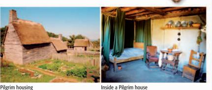
This reconstruction of the Plymouth settlement shows how the settlers built their homes: a simple wooden frame covered with wood slats and roofed with thatch kept out the worst of the elements
