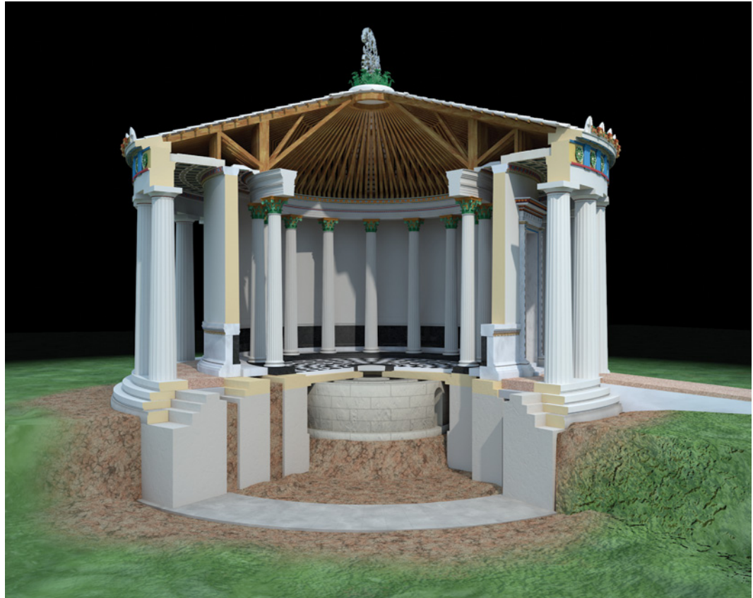
12.2 Reconstruction of the thymele (tholos) at Epidauros, designed by Polykleitos the Younger, c. 360–330 BCE. 3D model: John Goodinson. Scientific advisor: John Svolos. Image courtesy of John Goodinson.
