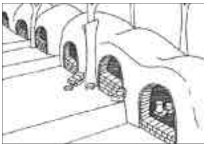
Figure 9. Celadons were fired in multichamber, tunnel-like kilns built along the side of a hill.
