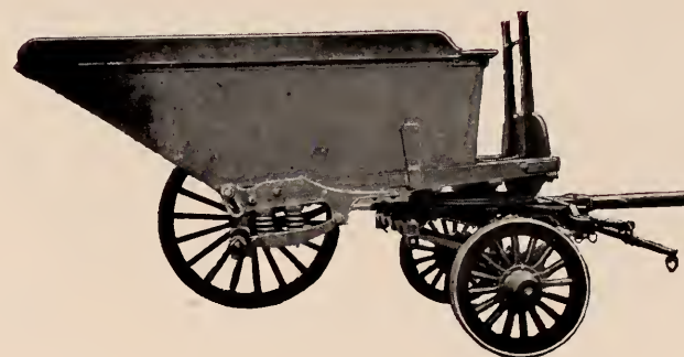
No. 13. View showing construction of spring pedestals
