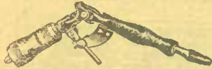
Angular Bit Stock, to be used in connection with any brace for boring in corners, $2.
