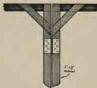
Detail of corner construction
