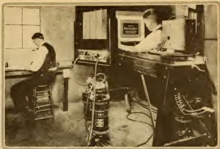
Here is the sub-titling department where the lines you read on the screen are photographed. These subtitles are "set up" in type and printed on a heavy piece of paper. They are then photographed.
