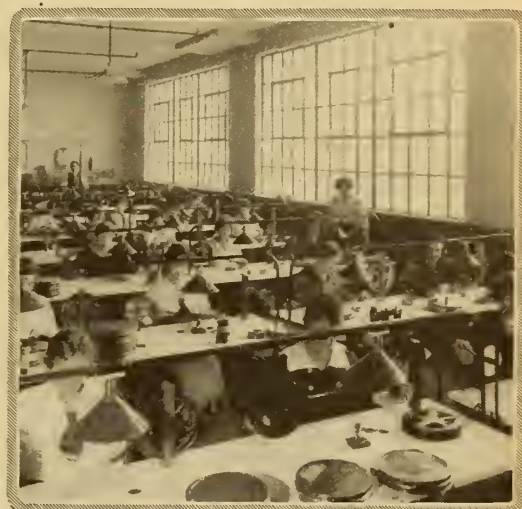
After the strips of positive film are developed, they go to the assembling room, where nimble-fingered young ladies put them together. Extreme care must be exercised to see that the strips are pasted in their proper places.
