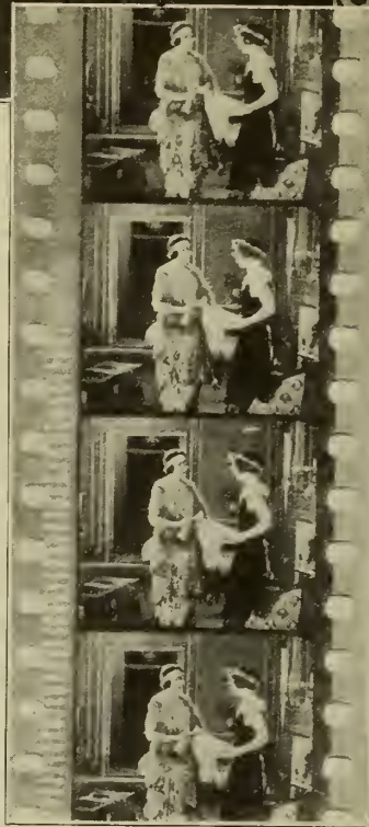
A section of the Phonofilm with the action and voice photographed together. The sound reproduction is contained in the parallel lines, which may be seen at the left of the film
