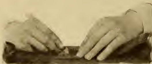
2—After the film is trimmed the operator uses a safety file to scrape the gelatine coating off the overlap as the gelatine would not permit the glue to stick.
