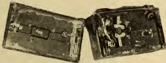
The Cine-Kodak after its immersion in the waters off the French coast
