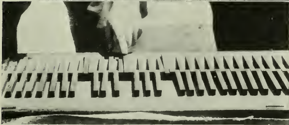
This is no piano, but it played a tune of death—movie death. This keyboard controlled the firing of seventy cannon. Electrically operated, it could fire a gun from any part of the ship
