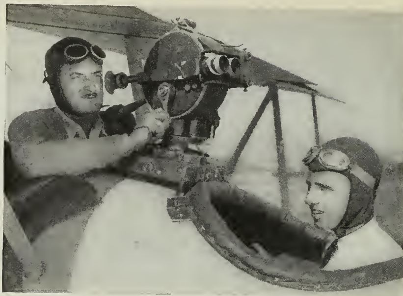
How those high-flying close-ups are filmed. The man with the camera is Le Roy Greiner, specialist in air photography. The camera is anchored firmly over the cockpit on a special stand, to keep it steady in spite of the terrific speed of the plane. This particular scene was filmed for Junior Coghlan's picture, "Marked Money"
