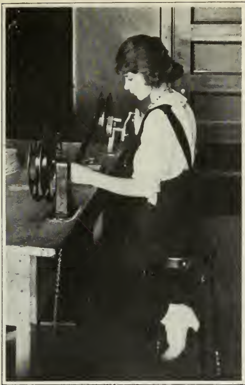
This is "Little Mabel, the Film Inspector." She inspects the reel to see that it is in good condition before it is sent out to the exhibitor. Every reel is inspected after every run. Mabel gets $25 a week for looking at pictures. She inspects about 100 reels a day. There are sixteen exposures to the foot of film, so Miss Mabel passes on 1,600,000 picture frames daily for Mutual.
