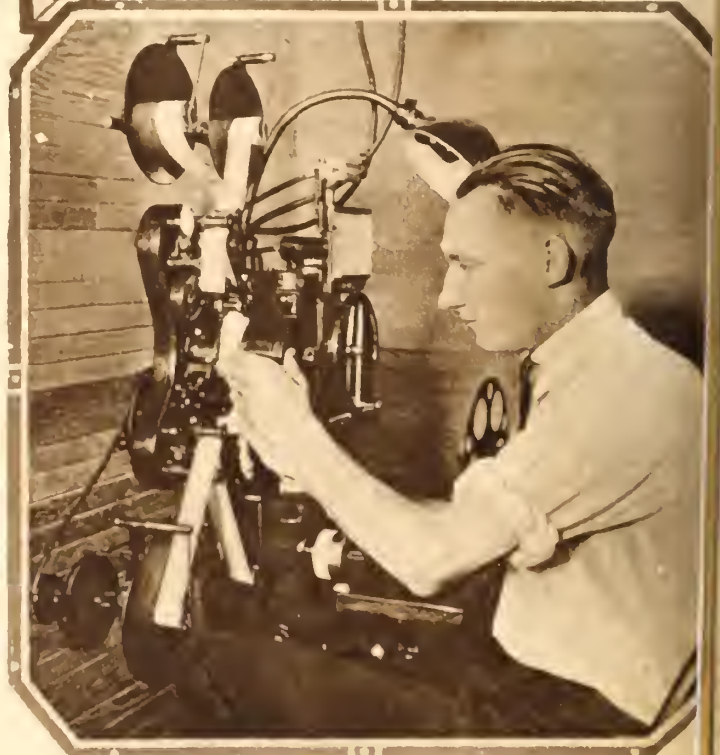
Below: A film printing machine, showing negative and positive sections in position.
