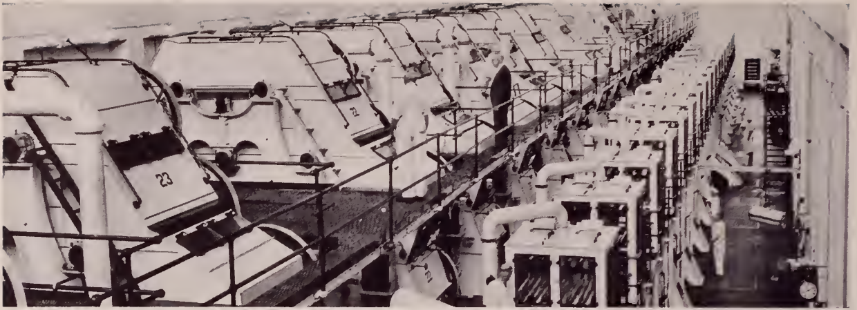
These machines convert fluid "dope" into endless sheets of the familiar transparent film base, which is very nearly invisible as it passes over the polished rollers.
