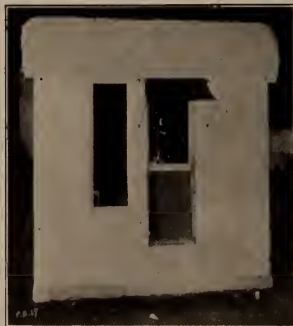
Sound-proof box in which talking picture cameramen work at Universal studio. The "refrigerator" prevents the noise of the camera reaching the microphone.
