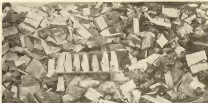
After the "cart-wheels" have been split. Note roughly shaped last blocks, in center of pile, that have just come through the mill.
