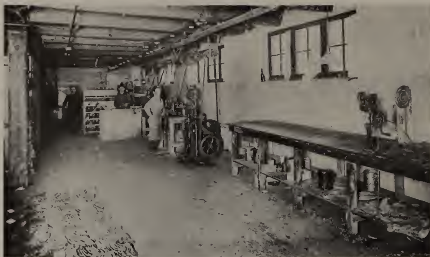
The sole room in the Lady Belle factory is on the ground floor of the building. Here the leather is cut to shape, rounded, channelled, tempered, and then sent to the lasting room.
