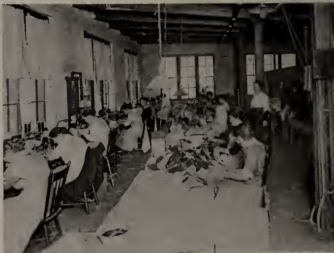
The upper stitching room in the Lady Belle plant is well equipped with daylight and, when artificial light is necessary each operator has an individual gooseneck electric fixture
