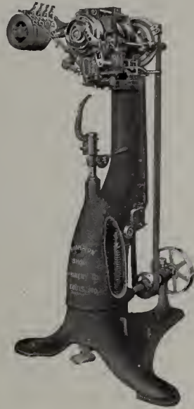
Champion combination clincher, fastener and heel slugging machine, installed in Neill Store at Peterboro
