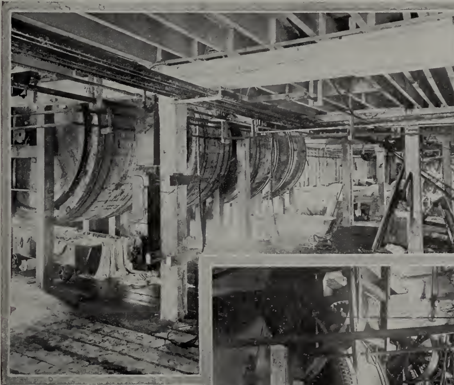
Drum tanning at Laing St. factory No. 2
