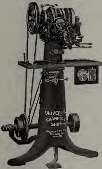
Universal Model Curved Needle and Awl Shoe Stitcher — heated by gas, gasoline, or electricity.
