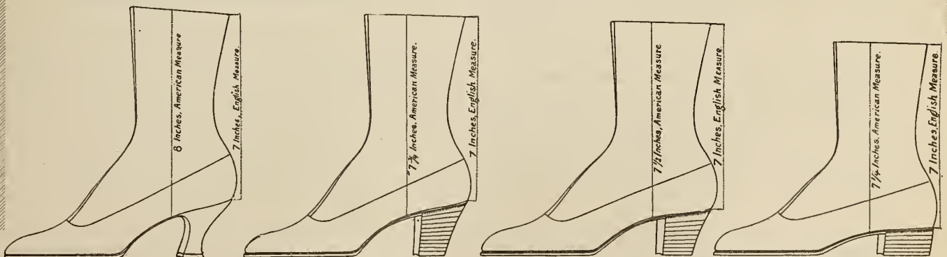
Illustrating the American and the English Methods of Measuring the Height of Shoes
