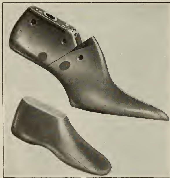
THE LOWER LAST IS ONE MADE FIFTY-FIVE YEARS AGO, THE OTHER IS ONE OF THE VERY LATEST HINGE LASTS
