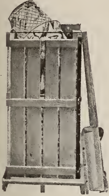
Waste paper bin and baler combined
