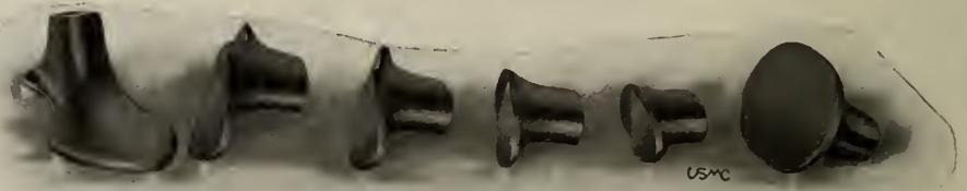
Five Well-Shaped Lasts and Beating-Out Block
