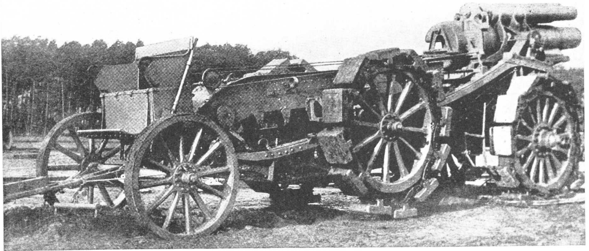
A powerful German siege gun transported by the use of caterpillar wheels. It was her advantage in heavy guns that gave Germany easy victory over Belgian forts.
