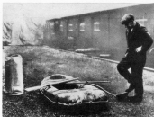
(5) Boat being inflated by foot pump.
