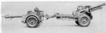
FIGURE 72.—25-pounder field gun-howitzer, Mk. II, on 25-pounder carriage, Mk. I (stowage position).
