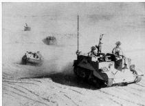
FIGURE 31.—Universal powered carrier fitted with 30mm gun on anti-aircraft mount and with Boys anti-tank rifle.
