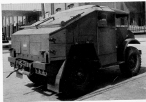
FIGURE 105.—Morris CA tracked field artillery tractor (model of use).
