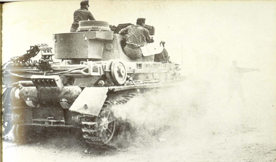
ABOVE: A PzKpfw IV Ausf D during the January 1942 offensive, showing the rear smoke emitter and a plain white outline type cross (IWM-MH5553).
