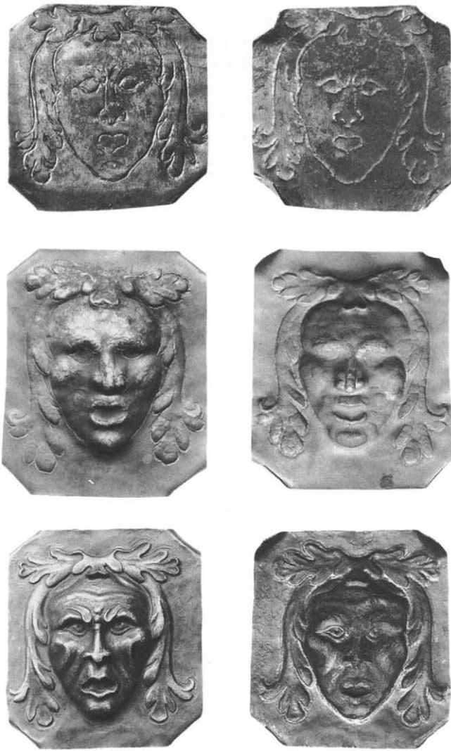
Figs. 32–37. The technique of embossing, illustrated in plates made by Leonard Heinrich, Armorer, Metropolitan Museum of Art, ca. 1940. The left column shows the exterior of each plate, the right column the interior. The pattern is first incised with chisels on the exterior (fig. 32), after which the plate is turned over and set face down into a bed of pitch and the relief is bossed out with hammers (fig. 35). Finally the outer face is chased with chisels and punches to give definition to the relief (figs. 36, 37)
