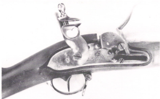
Lock of the 'new' Prussian musket of 1809, as manufactured at Neisse in Upper Silesia. Note the shield around the pan, protecting the priming from the weather, and the firer's face from the flare of the priming.
