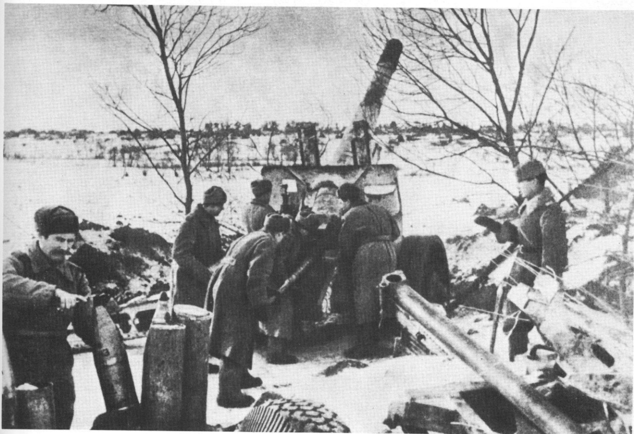
76. The standard Soviet heavy field gun of the war was the ML-20 152mm Model 1937; the self-propelled versions were the SU-152 and ISU-152. This battery is in action outside Zytomierz in 1944.
