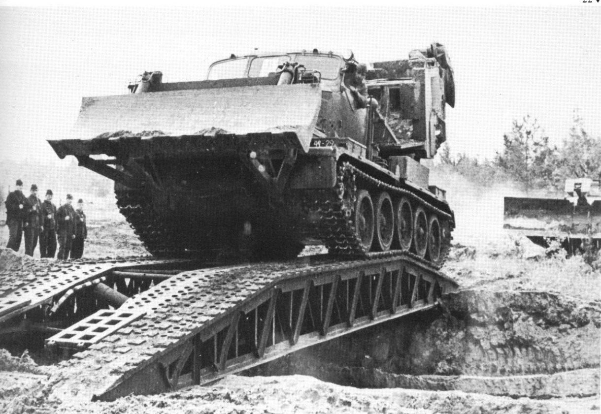
22. An MDK-2M ditching machine crosses a tank-laid bridge. These vehicles are used to dig anti-tank ditches or defensive positions, and this particular example belongs to the Tyumen Higher Engineer Command School.
