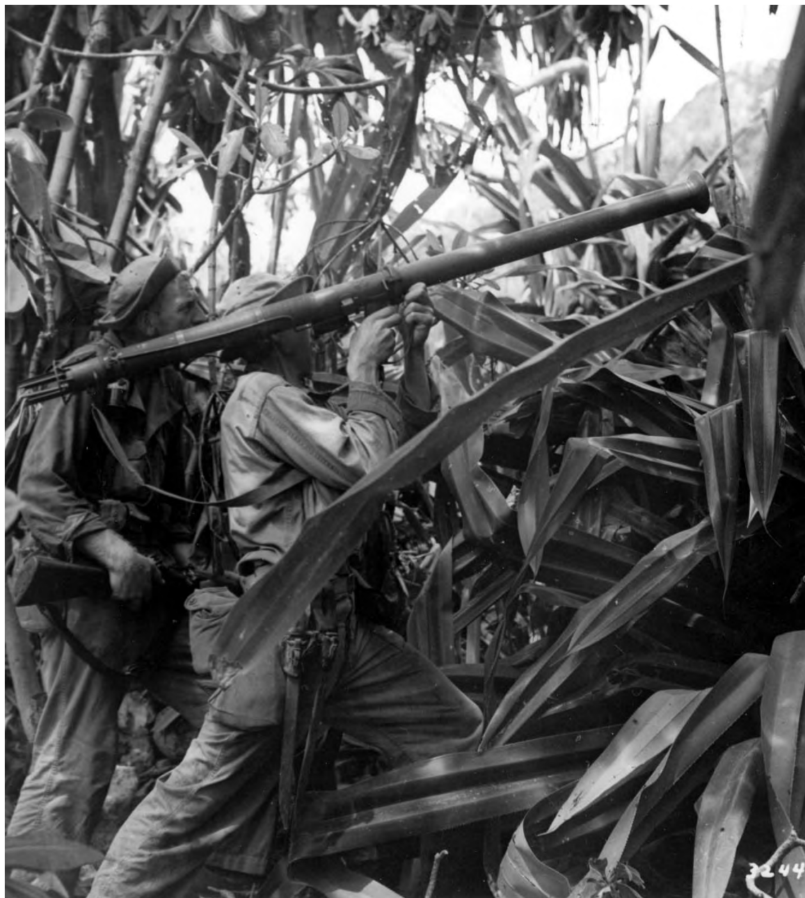
2.36-INCH ROCKET LAUNCHER M9 being fired into a cave on Saipan, 28 July. These launchers, called bazookas, were usually equipped with a flash deflector to protect the operator from unburned powder as the rocket left the tube. The bazooka was employed against tanks, armored vehicles, pillboxes, and other enemy emplacements. Operations to rid the island of the enemy continued for nearly two months after organized fighting had ceased.
