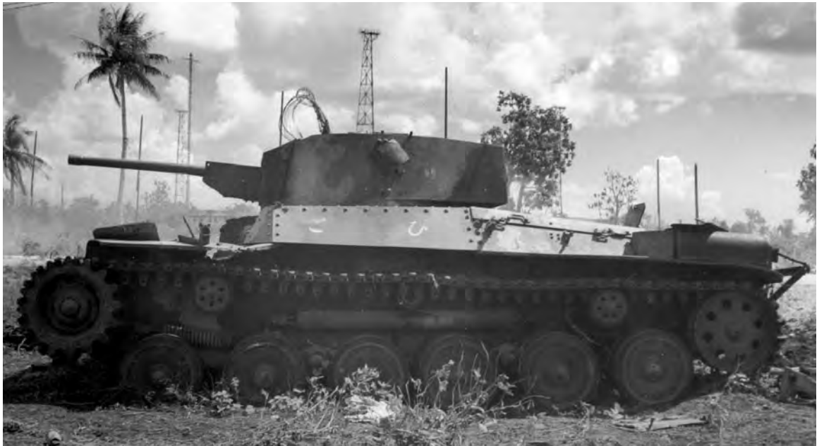
CAPTURED ENEMY EQUIPMENT ON SAIPAN. Type 93, 13.2-mm. machine gun mounted on a naval-type pedestal, dual-purpose single mount, which could be used emplaced on a dual-purpose position or emplaced solely for antiaircraft fire or only for ground fire (top). A Type 97 medium tank mounting a 47-mm. tank gun and weighing 15 tons; its manually operated turret could be traversed 360 degrees (bottom).
