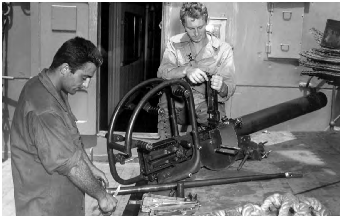
ABOARD A TROOPSHIP, 14 December 1943, en route to invade New Britain on Arawe. Infantryman relaxes on a cork life raft (top) while two men check and reassemble a flexible, water-cooled .50-caliber Browning machine gun M2 (bottom). While Army and Navy bombers pounded Rabaul, landings were made on Arawe peninsula on the southern coast of New Britain, 15 December 1943.
