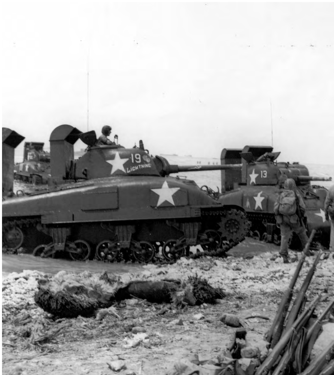
MEDIUM TANKS M4A1 WITH 75-MM. GUNS, going ashore on Kwajalein. The stacks, at the rear of the tanks, were used to extend the vented openings; unvented openings were sealed with tape and sealing compound to render the hulls watertight. Waterproofed vehicles could be operated satisfactorily in water deeper than otherwise possible, permitting them to wade in from landing craft halted at greater distances from shore.
