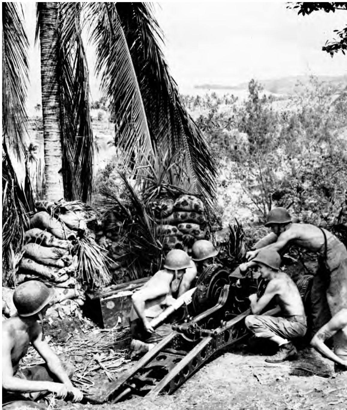
MARINES ON GUADALCANAL in October 1942 firing a 75-mm. pack howitzer M1A1 mounted on carriage M8. Although this weapon was primarily used for operations in mountainous terrain, it was capable of engaging antitank targets.
