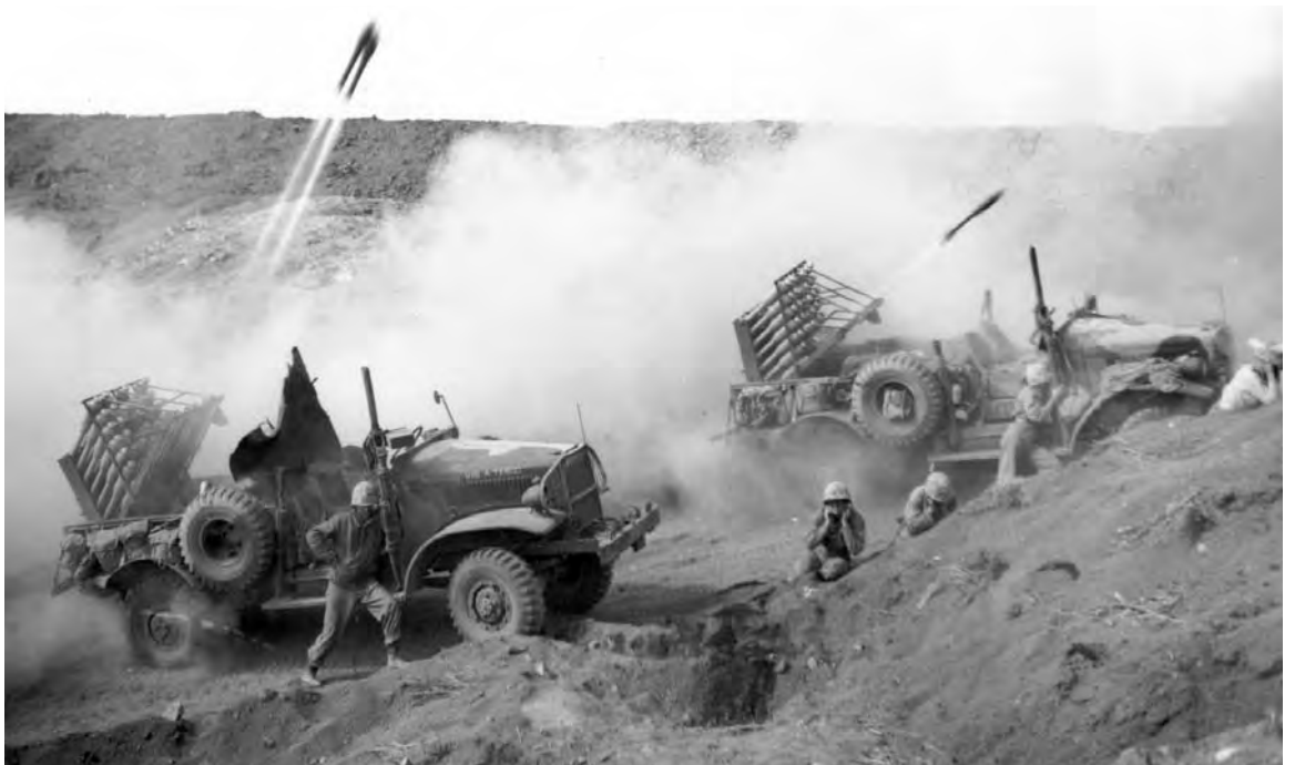
75-MM. GUN MOTOR CARRIAGES M3 FIRING at enemy positions on Iwo Jima (top). 4.5-inch automatic rocket launchers T45 mounted on two \frac{3}{4} -ton trucks, firing; this gravity-feed automatic launcher was developed as a Navy standard item for firing the 4.5-inch Navy barrage rocket (bottom)
