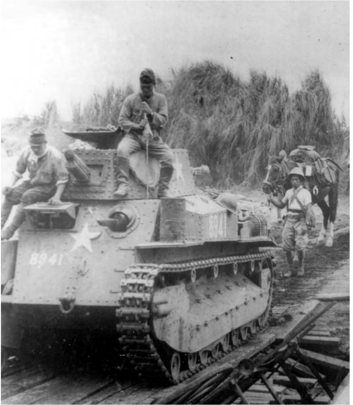
JAPANESE ADVANCING during the drive on Manila. The medium tank is a Type 94 (1934), with a 57-mm. gun with a free traverse of 20 degrees right and left. It had a speed of 18 to 20 miles an hour, was manned by a crew of 4, weighed 15 tons, and was powered by a diesel engine.
