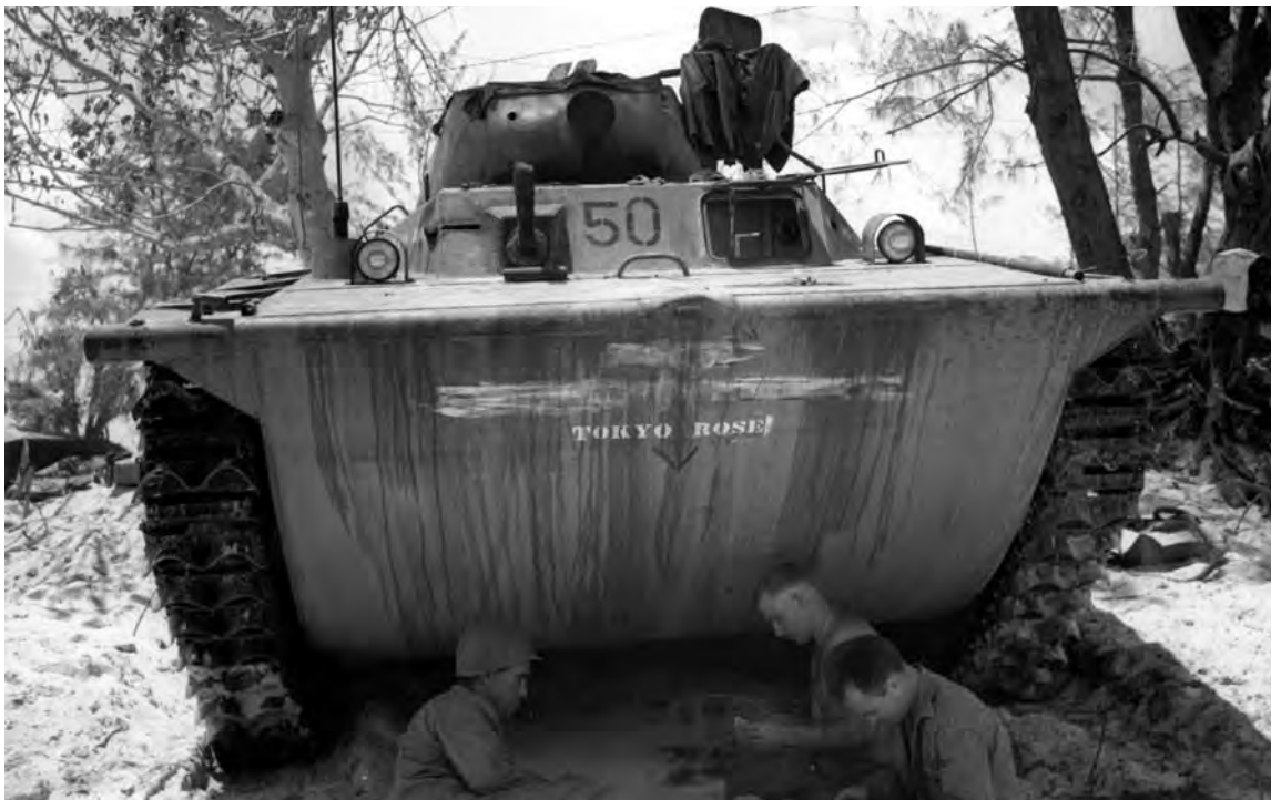
TRACTOR TOWING A 155-MM. GUN OVER A PONTON CAUSEWAY reaching from an LST to shore on Saipan. The tractor is a high-speed 18-ton M4 model; the 155-mm. gun M1A1 is mounted on an M1 carriage (top). A landing vehicle, tracked, provides a shady spot for a game of cards during a lull in the fighting; this armored amphibian LVT (A) (4) was the same as the LVT (A) (1) except for an M8 75-mm. howitzer turret which replaced the 37-mm. gun (bottom). On Saipan tanks and heavy artillery added the weight of their guns to renewed naval gunfire and aerial bombardment after the Battle of the Philippine Sea.
