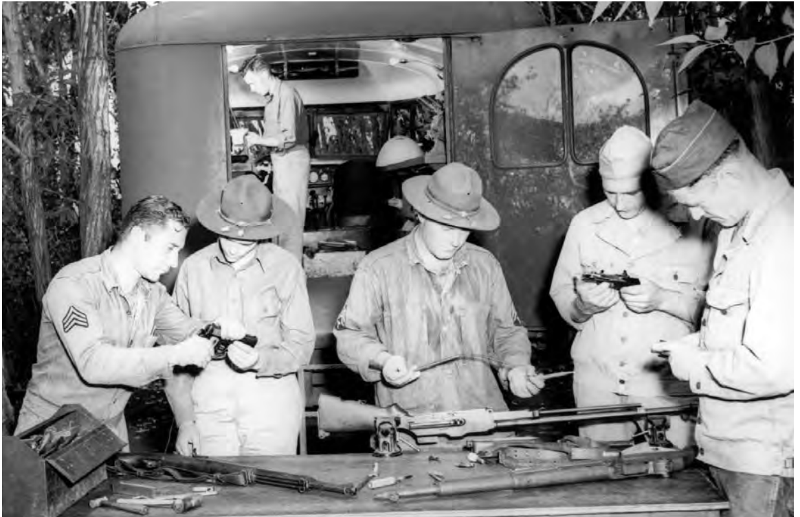
A BATTERY OF 105-MM. HOWITZERS M2A1 firing during maneuvers (top); ordnance men repairing small arms (bottom). Two men are holding .45-caliber automatic pistols M1911; in the vice on the table is a .30-caliber Browning automatic rifle M1918A2; on the table are two .30-caliber rifles M1.
