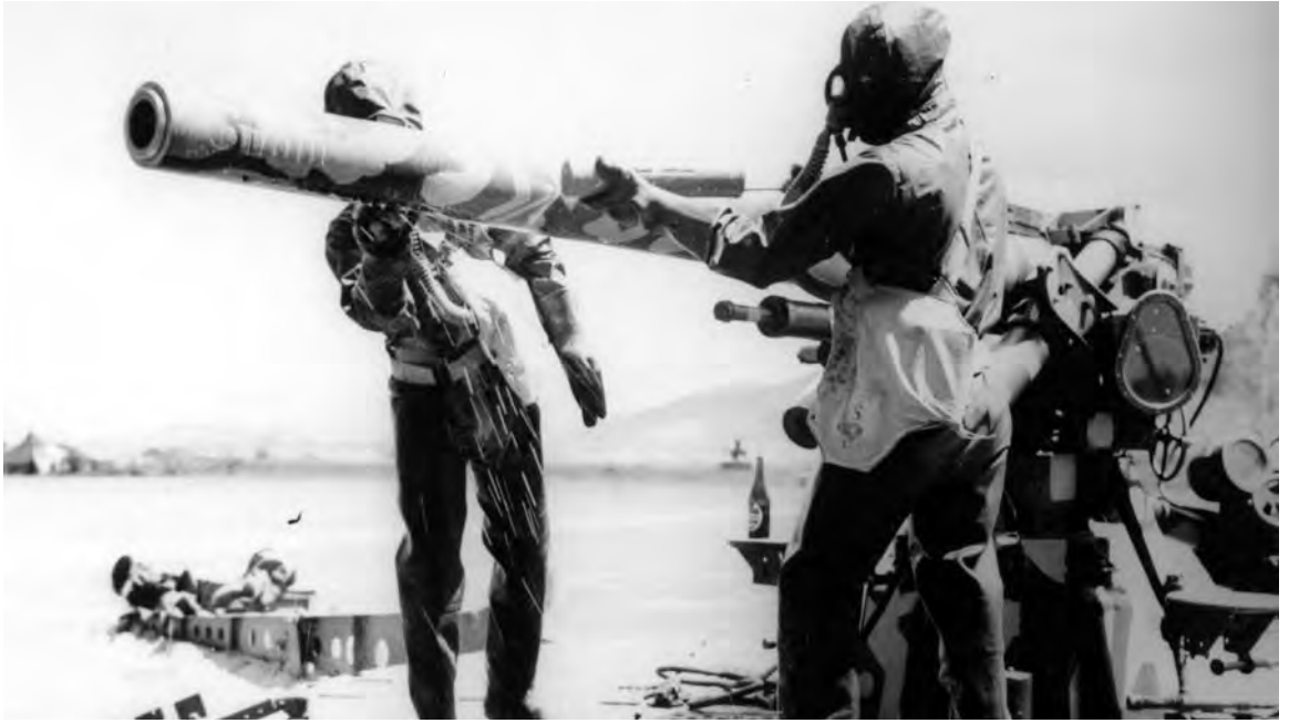
3-INCH ANTI-AIRCRAFT GUN M3 being decontaminated by members of a coast artillery battery after the gun had been subjected to mustard gas during training in chemical warfare (top). After firing, artillerymen open the breech of their 155-mm. howitzer M1918 mounted on an M1918A3 carriage (bottom).
