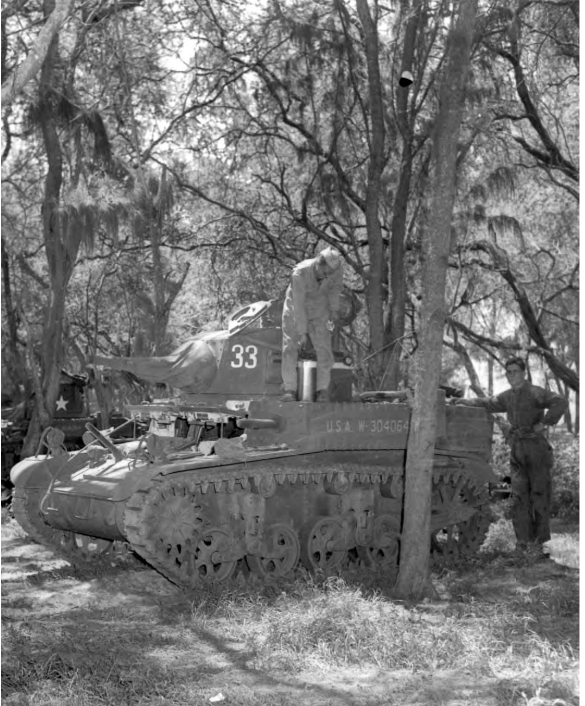
LIGHT TANK M3 being refueled during jungle maneuvers. This tank, which replaced earlier light tank models, had as its principal weapon a 37-mm. gun.
