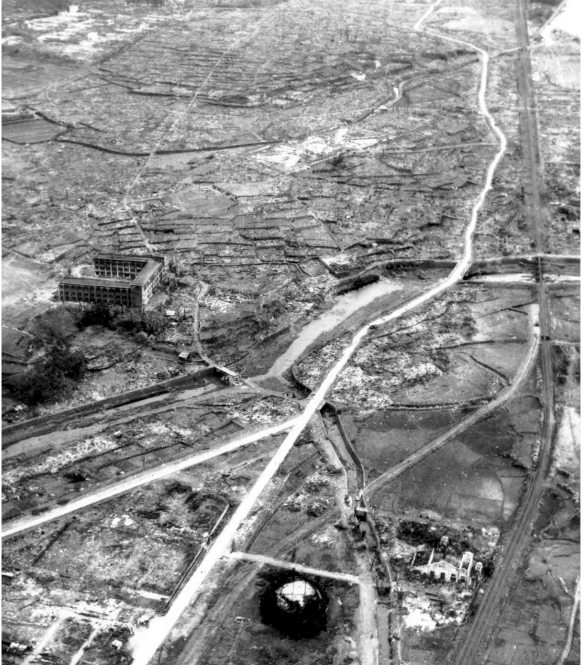
DAMAGE AT NAGASAKI, showing large areas where most of the buildings were leveled. Buildings constructed of reinforced concrete suffered less than other types. The circular structure, at lower center, is the Ohashi Gas Works, approximately 3,200 feet north of ground zero. The concrete building at left center is the Yamazato School, approximately 2,300 feet north of ground zero.
