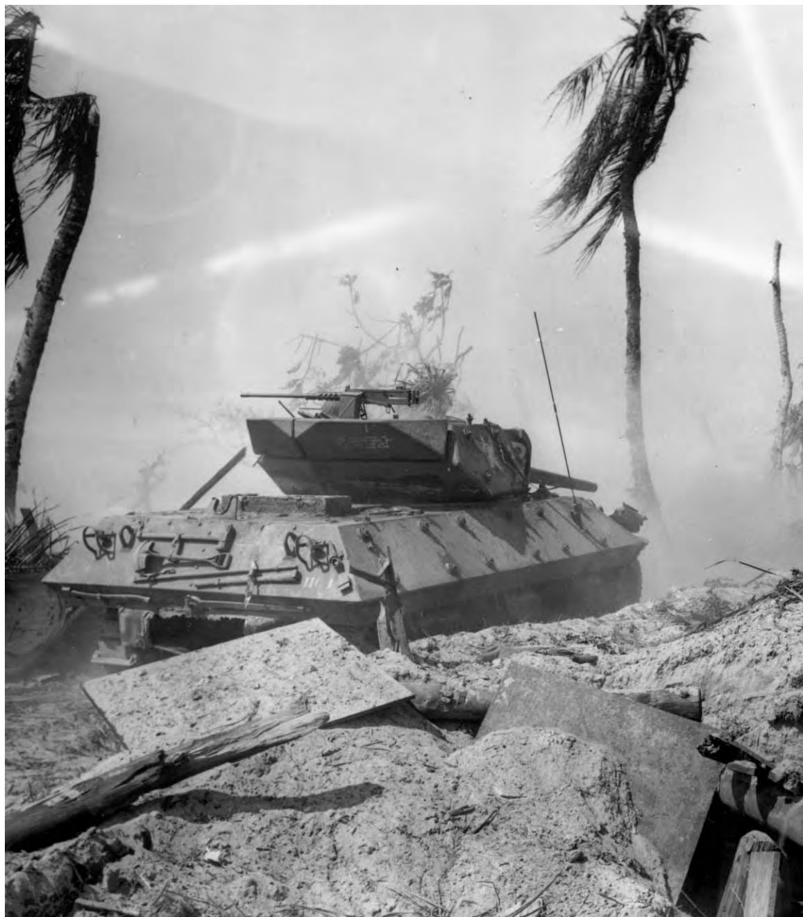
GUN MOTOR CARRIAGE M10, used to blast pillboxes on Kwajalein. This weapon, called a tank destroyer, was mounted on the medium tank chassis and had a 3-inch gun M17 in a semiopen turret, and a .50-caliber machine gun at the rear of the turret for protection against low flying planes. Six days after the main landings had taken place, Kwajalein was in U.S. hands.
