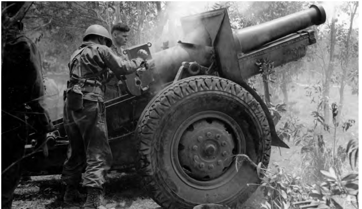
3-INCH ANTI-AIRCRAFT GUN M3 being decontaminated by members of a coast artillery battery after the gun had been subjected to mustard gas during training in chemical warfare (top). After firing, artillerymen open the breech of their 155-mm. howitzer M1918 mounted on an M1918A3 carriage (bottom).
