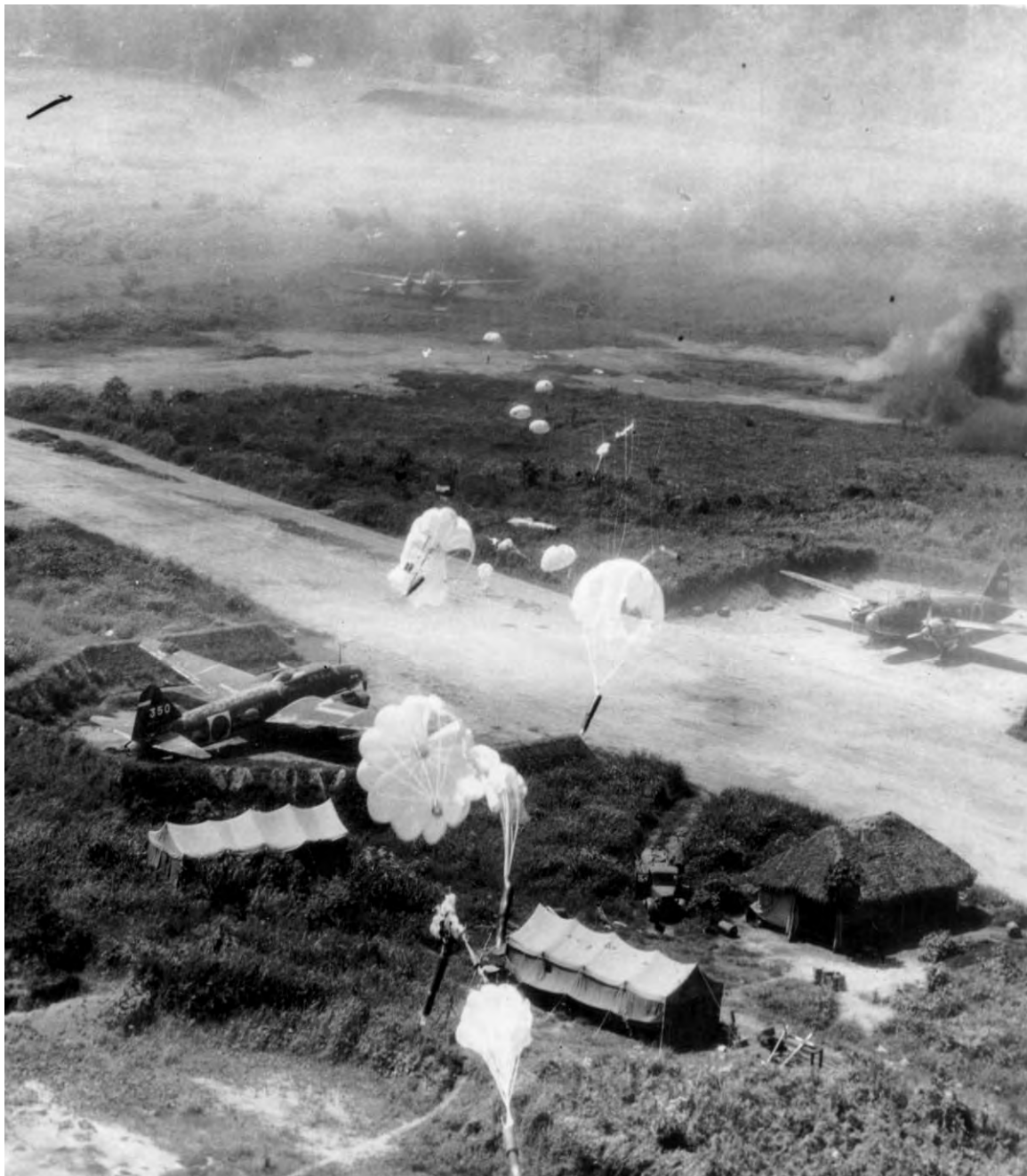
PARACHUTE BOMBS dropping from low-flying American planes during a raid over Rabaul. Parachute bombs were used to prevent self-destruction of the attacking low-flying bombers by the blasts of their own bombs. It was claimed that more than 200 enemy aircraft were destroyed or damaged on this raid, in addition to other materiel, ships, and installations.
