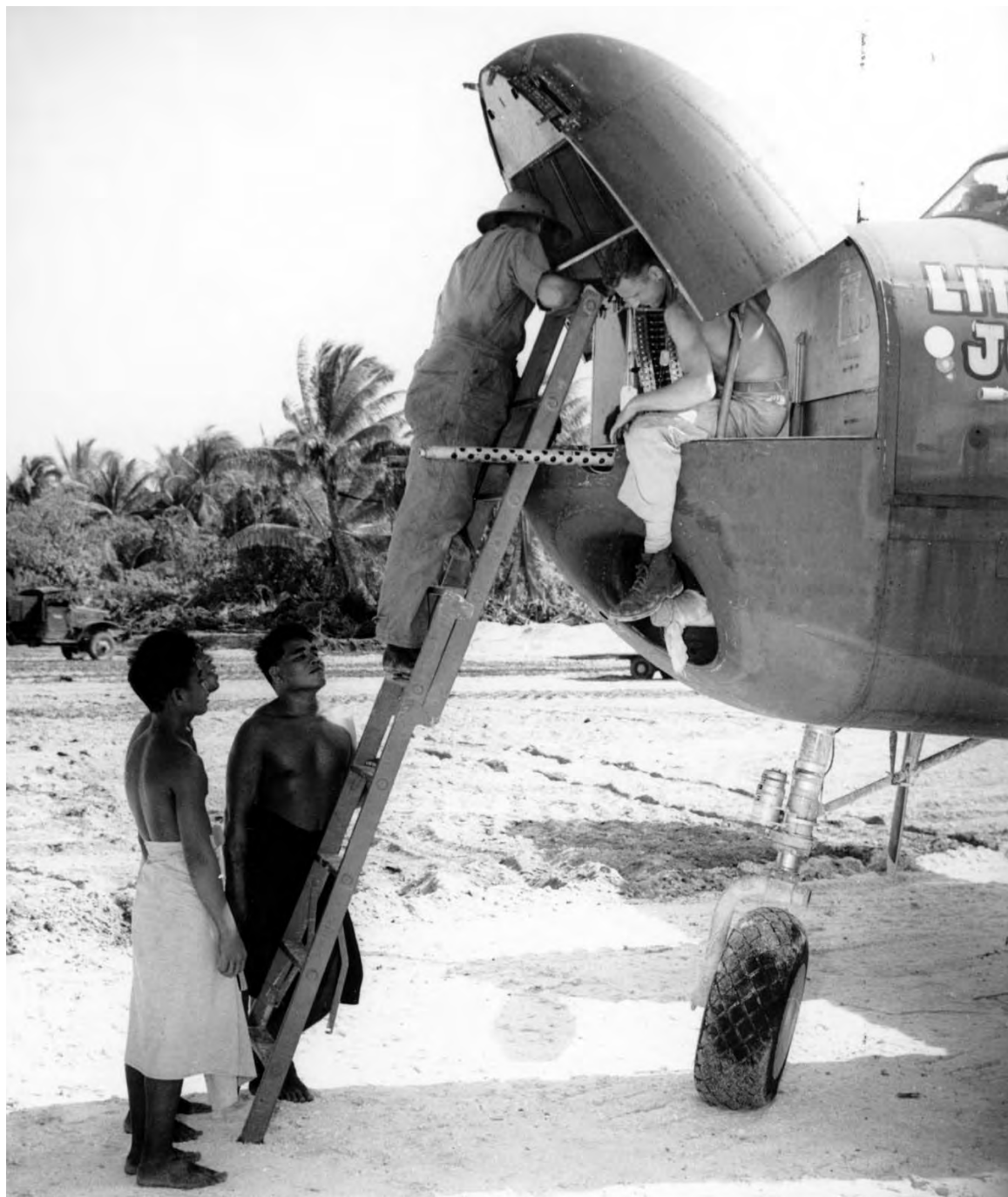
ARMORERS place a .50-caliber aircraft Browning machine gun M2A1 in the nose of a North American B-25 at the airfield on Betio Island as interested natives look on. This gun was considered one of the most reliable weapons of the war.
