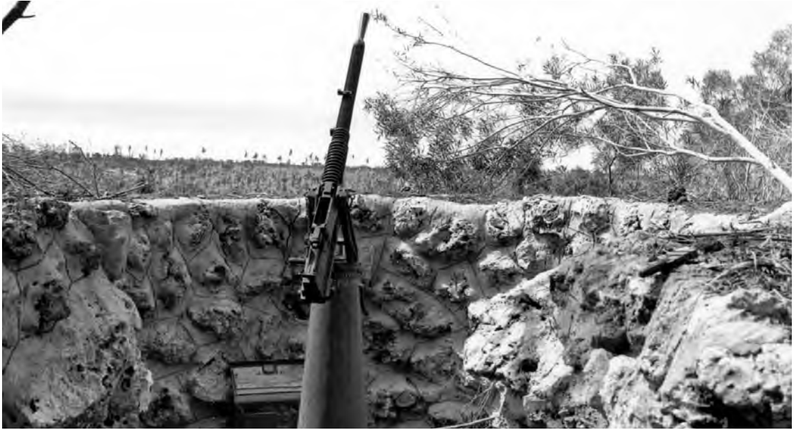
CAPTURED ENEMY EQUIPMENT ON SAIPAN. Type 93, 13.2-mm. machine gun mounted on a naval-type pedestal, dual-purpose single mount, which could be used emplaced on a dual-purpose position or emplaced solely for antiaircraft fire or only for ground fire (top). A Type 97 medium tank mounting a 47-mm. tank gun and weighing 15 tons; its manually operated turret could be traversed 360 degrees (bottom).
