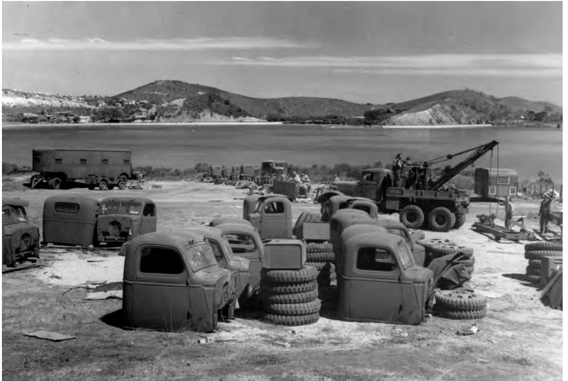
MEN OF AN ORDNANCE UNIT ASSEMBLING VEHICLES which had arrived crated in sections. By October 1942 twenty-five men were completing six vehicles a day on this assembly line.
