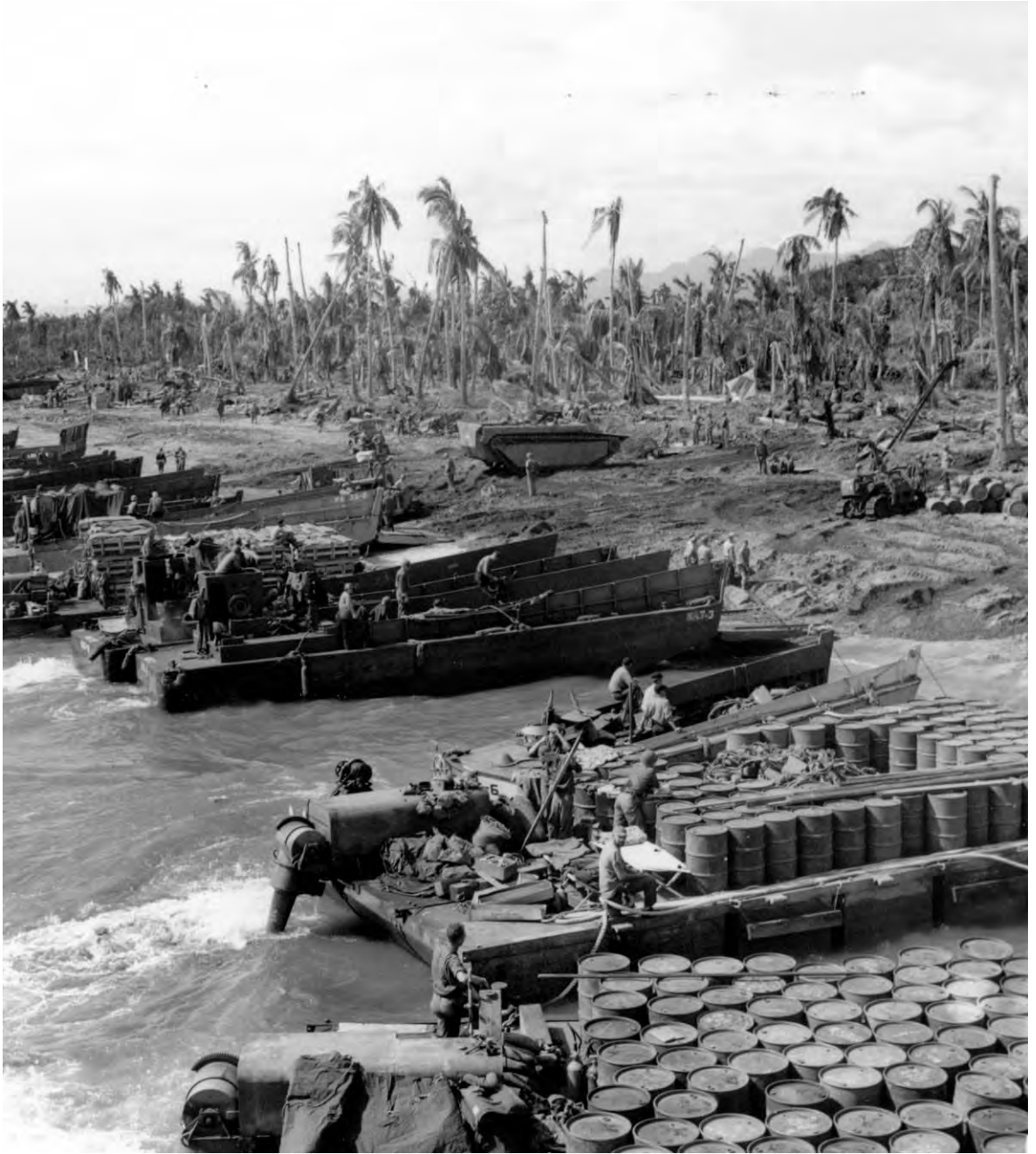
UNLOADING AT A BEACH ON LEYTE, 21 October 1944. Beyond the two barges are several LCM (3)'s. An LVT (A) (2), the armored Buffalo, can be seen on the beach. On 20 October landings were made on three beaches: one in the Palo area; another between San Jose and Dulag; and the third about fifty-five miles to the south to control Panaon Strait which was between Leyte and the near by island of Panaon.
