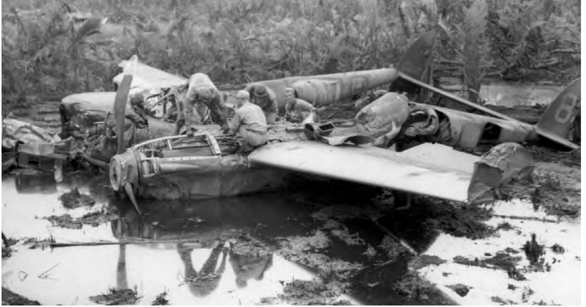
REMAINS OF A LIGHTNING FIGHTER PLANE P-38 which crashed during a landing (top), and a Flying Fortress B-17 which crashed when its right wheel gave way on an airstrip at Aitape (bottom). Since spare parts to maintain aircraft were difficult to obtain, maintenance men would strip crashed and crippled planes of usable parts almost before the engines cooled.
