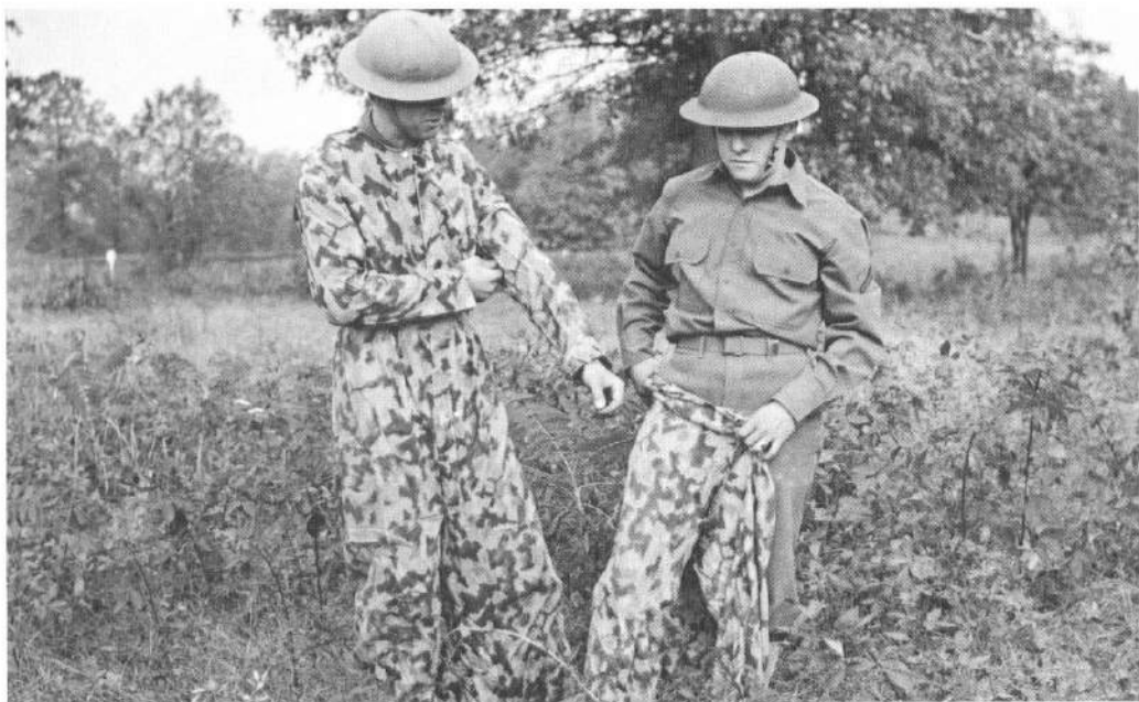
M1940 experimental suits of printed cotton and rayon camouflage design being tested by the Engineer Board at Fort Belvoir, Virginia, during 1941.
