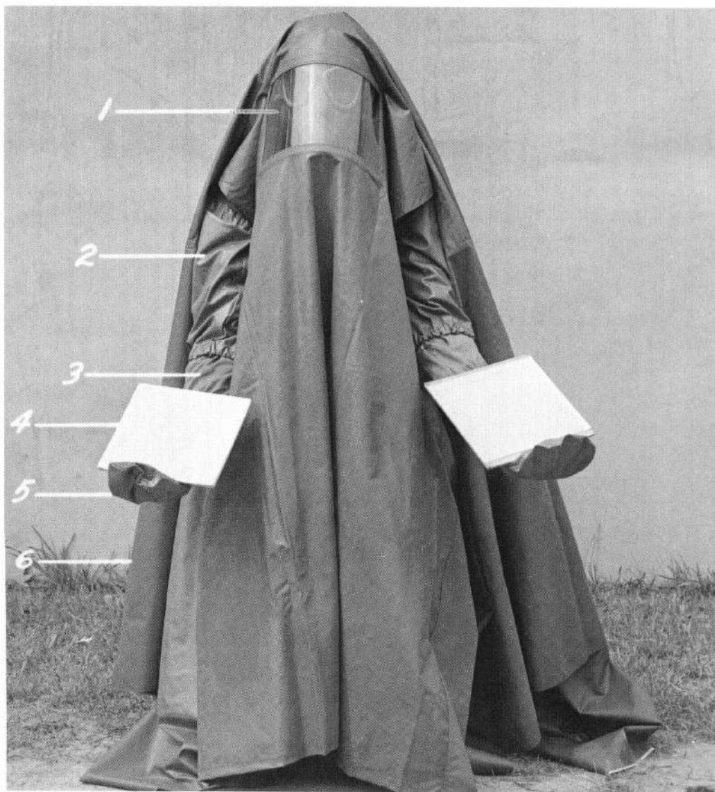
Army soldier in complete individual protective outfit during aerial-delivered mustard gas testing during June 1943: (1) transparent window, (2) impermeable sleeves, pulled down to show length and upper ends, (3) forearm protection, (4) panels to record Chemical Warfare Service spray results, (5) impermeable mittens, (6) impermeable individual protective cover.
