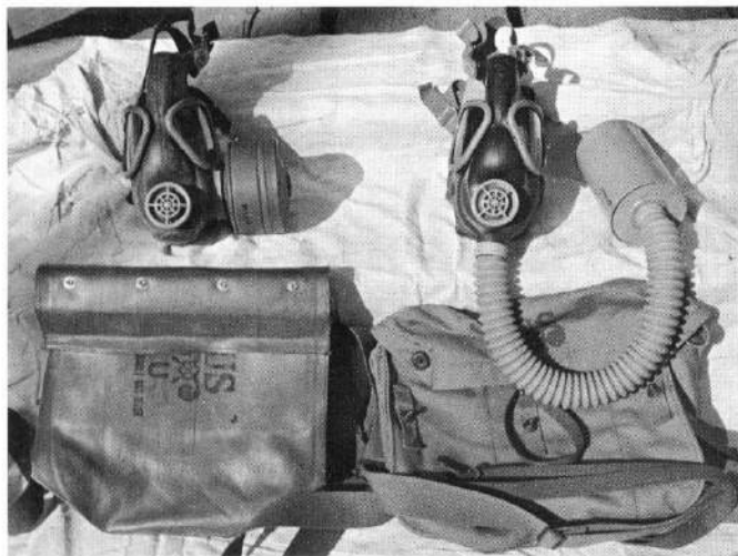
Actual items used for gas countermeasures during D-Day in June 1944 included this drum canister-equipped assault gas mask ( left , later designated the M5 combat service gas mask) with its waterproof carrier. It is contrasted with the M3 light-weight service gas mask and M10 canister ( right ), connected by the awkward hose that interfered with prone firing. Unfortunately, both neoprene "black rubber mask" types proved defective under winter fighting conditions.
