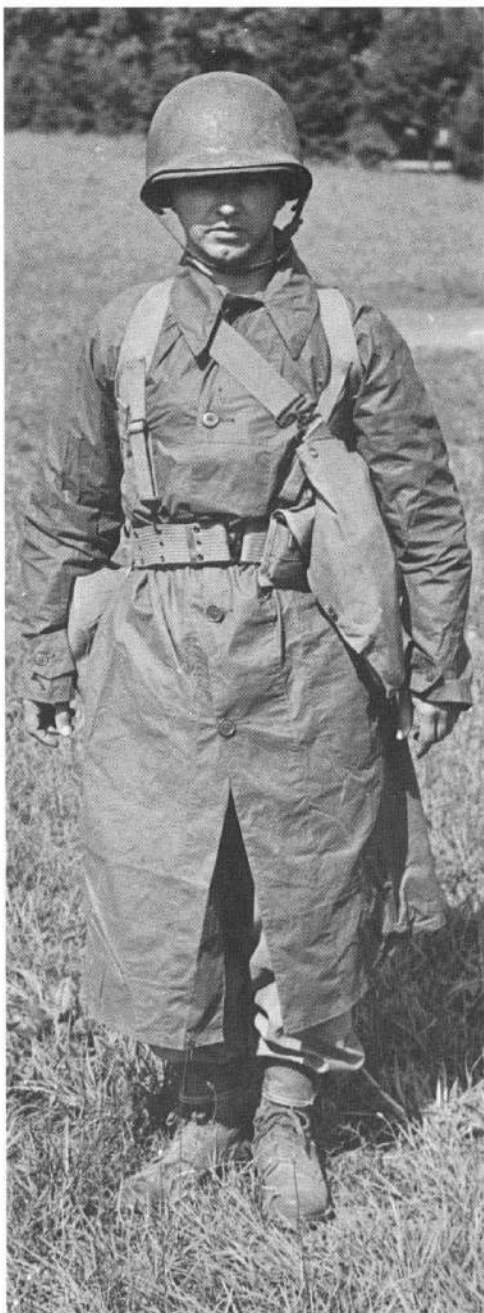
Experimental synthetic resin-coated raincoat of lengthened design worn with light individual combat equipment and gas-mask carrier during Quartermaster Board testing in early 1943.
