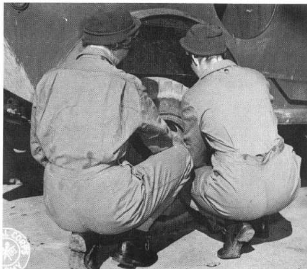
Bending movement also strained the back material on the women's one-piece work suit ( right ), often tearing buttons off the drop seat. The trousers of the two-piece suit ( left ) were unaffected by the same exercise.
