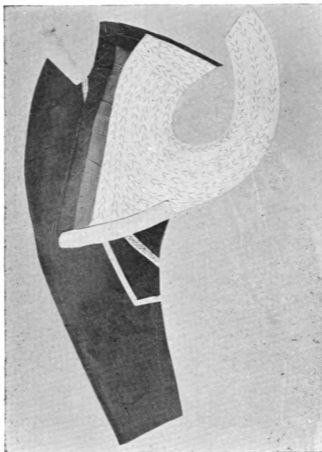
Diagram 7—Padding Stitches. This cut illustrates the correct method of putting in padding stitches as described in Section X.
