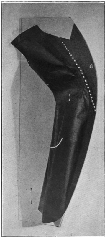
Diagram 15—This cut shows how the lapel is pressed into shape after the front edge has been cut away. Figure 4 shows the rounded effect secured on the edge of the lapel.
