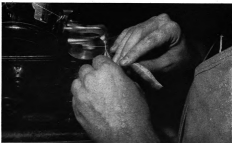
Fig. 9.—Position of operator's hands at machine, fine work.
