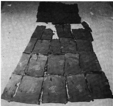
Fig. 33.—Close-up of cut coat skin layout on pattern (worked hair up).
