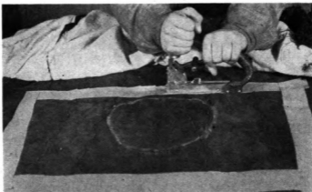
Fig. 145.—Stapling—in this instance for local nailing purposes. (See footnote on page 193.)
