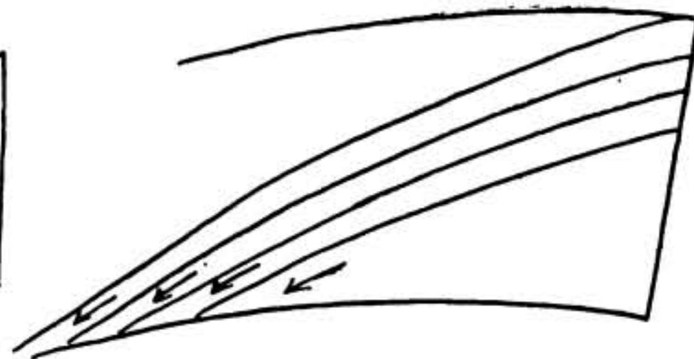
TECHNIQUE AND EFFECT OF "LET-IN STEP CUTS" - ARROWS SHOW HOW SLIGHT DRAWING OF STRIPS AIDED SHAPING
