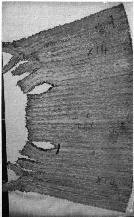
Fig. 130.—Typical appearance of leather side of let-out body—nailed muskrat coat.
