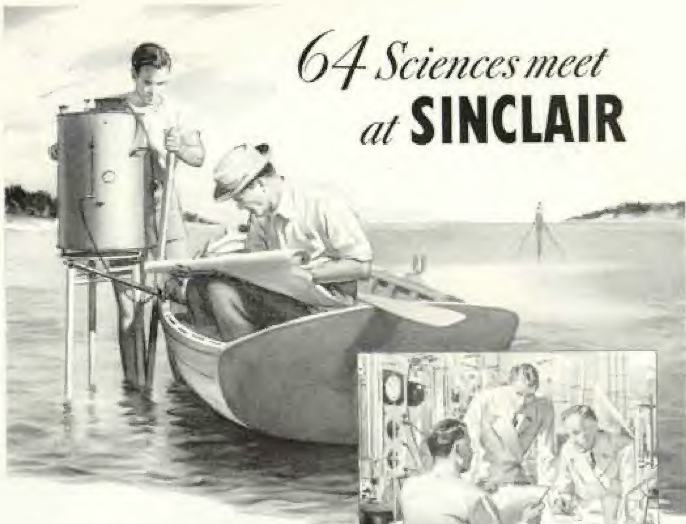
Geophysical exploration for oil extends even into the water. Here geophysicists are doing preliminary work with a gravity meter in the Gulf of Mexico.
