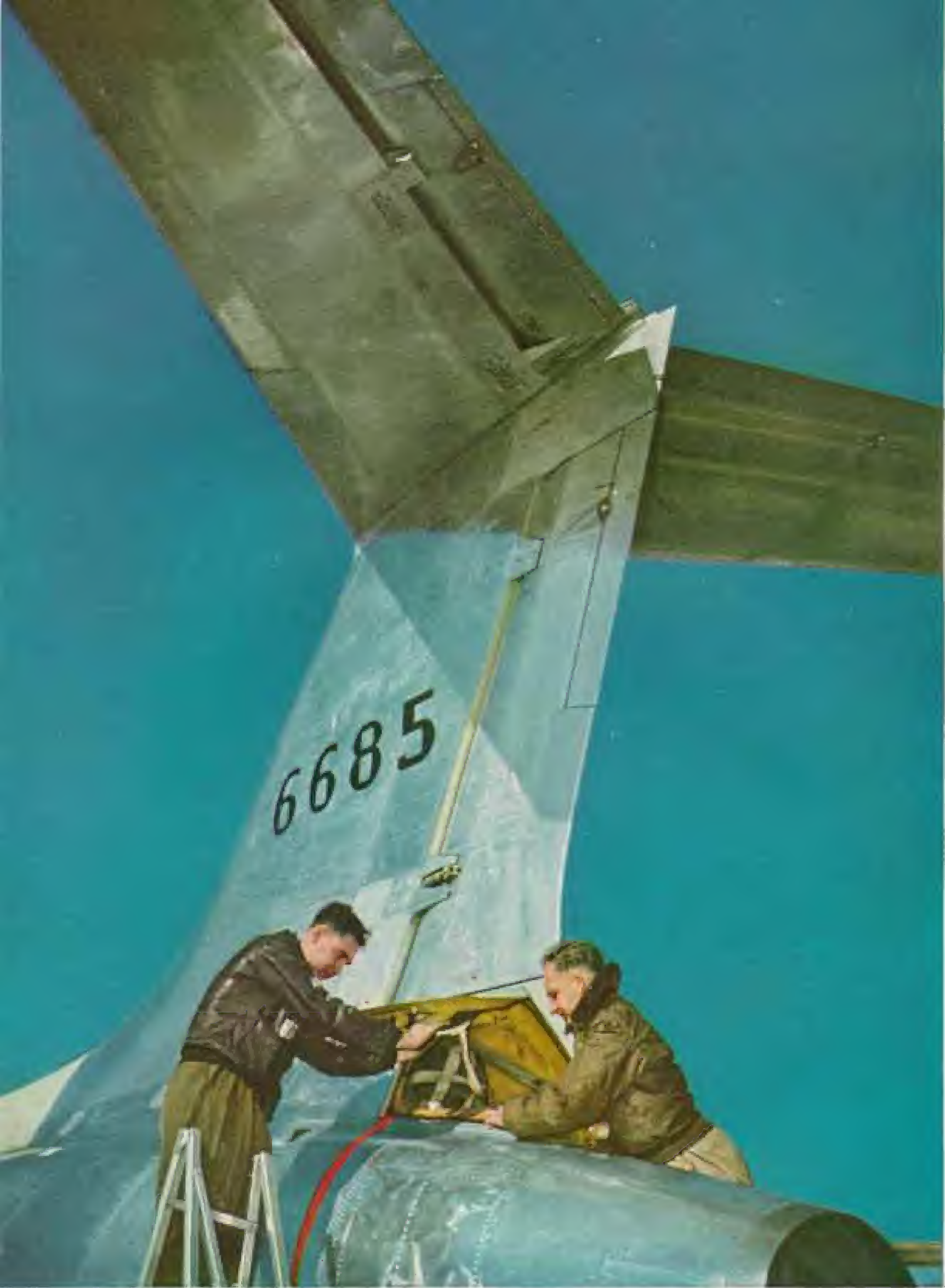
Behind the Towering "T" Tail, Crewmen Stow an XB-51 Jet Bomber's Parachute Brake For landings on small combat-area fields, the chute slows down this lightning-fast three-jet Glenn L. Martin bomber. The big, rakish, swept-wing speedster was designed for Air Force support of ground troops.
