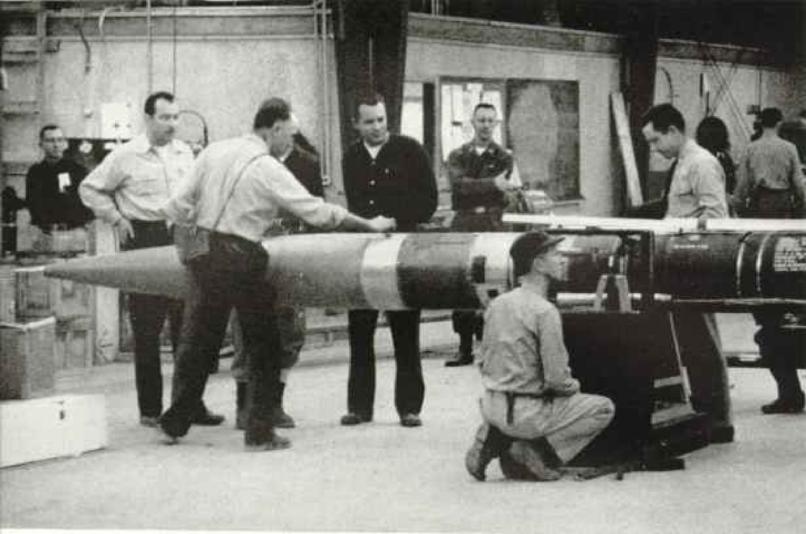
Scientists Weigh an Aerobee on Fore-and-aft Scales to Find Its Center of Gravity
