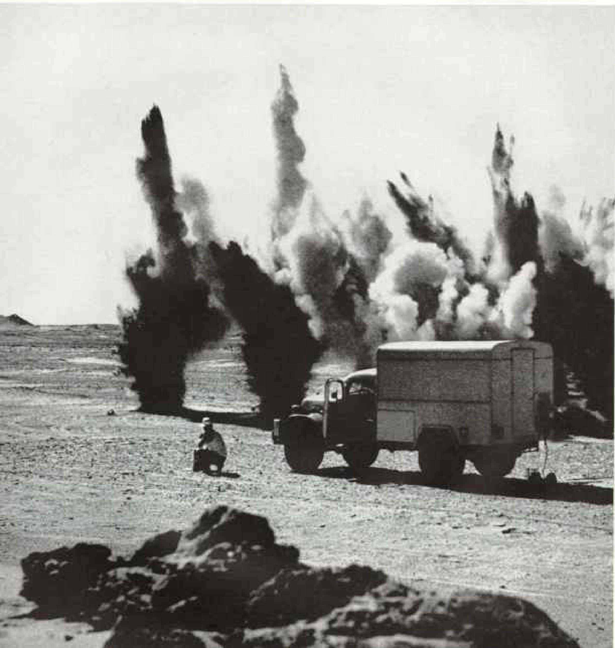
Dynamite Hurls Geysers of Sand Above the Desert as French Oil Geologists Sound
