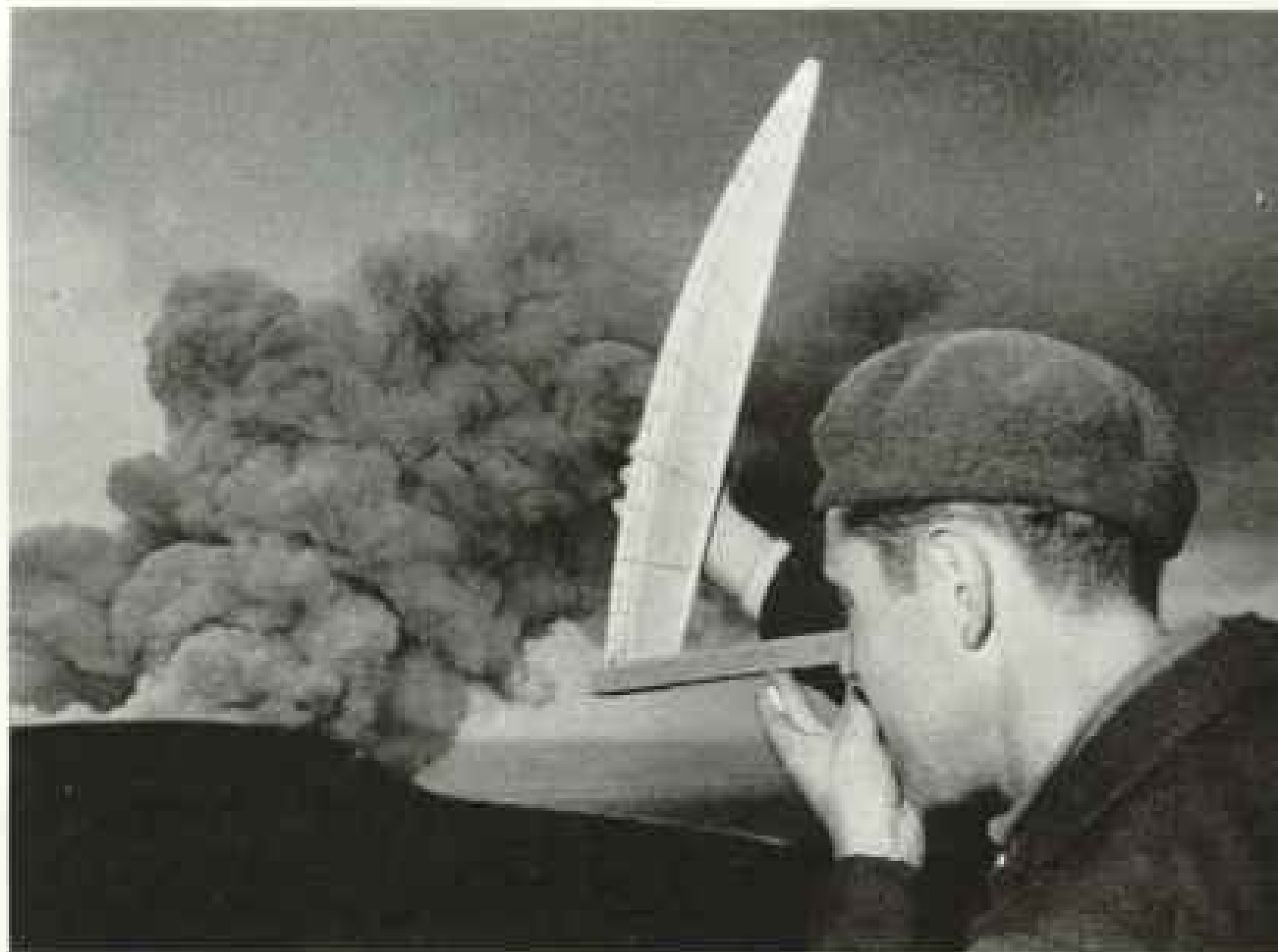
A homemade protractor helps Tomás Pacheco da Rosa estimate the eruption's height. An assistant lighthouse keeper at Capelinhos until flying rocks, earth tremors, and sulphurous gases closed the beacon, he has stayed on as the Portuguese government's official observer.
