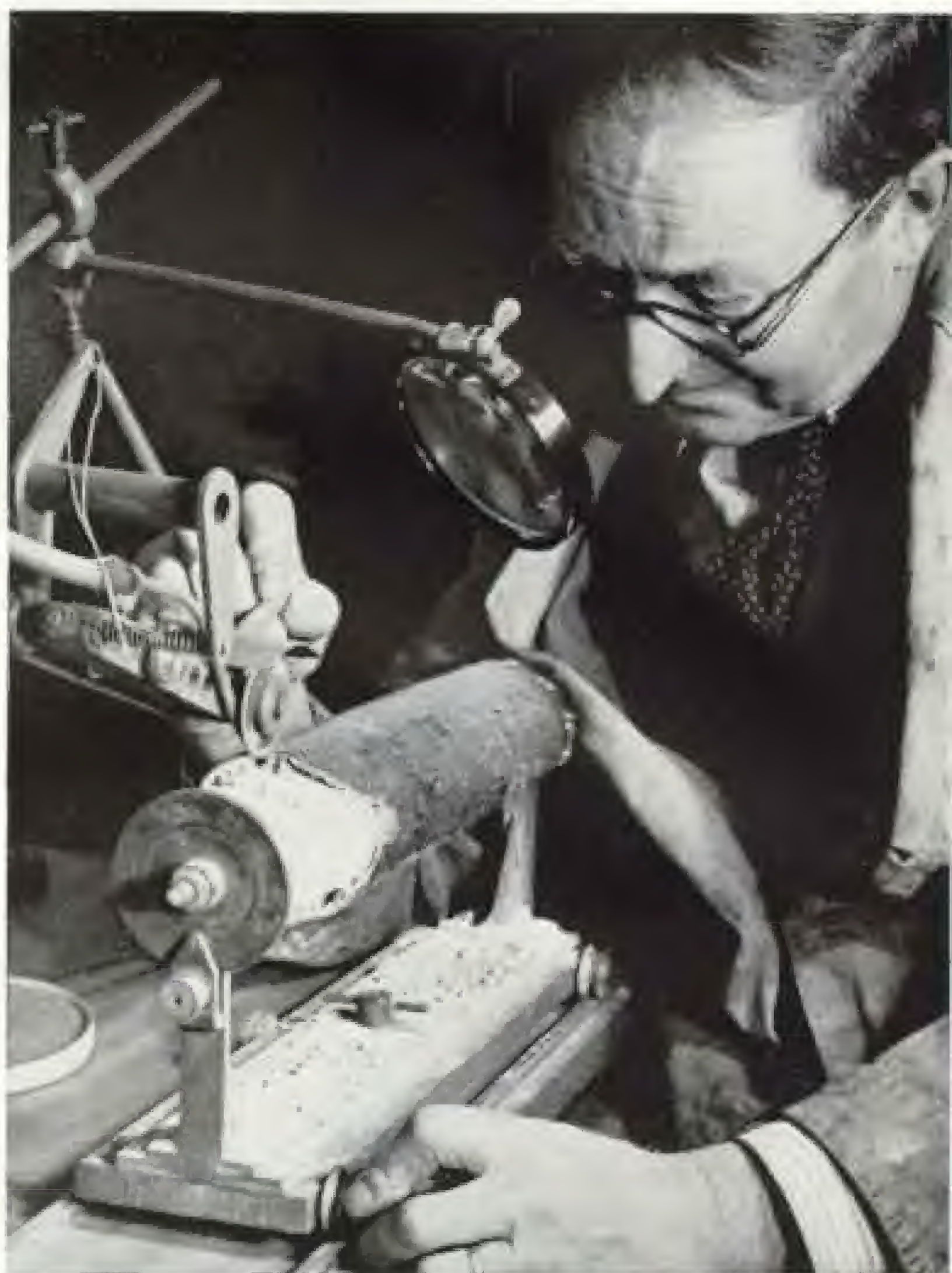
Ingenuity triumphs as H. Wright Baker of the University of Manchester, England, slices open the copper rolls with a specially adapted saw used to slit pen nibs. To prevent shattering, Professor Baker coated the surfaces with a plastic.
