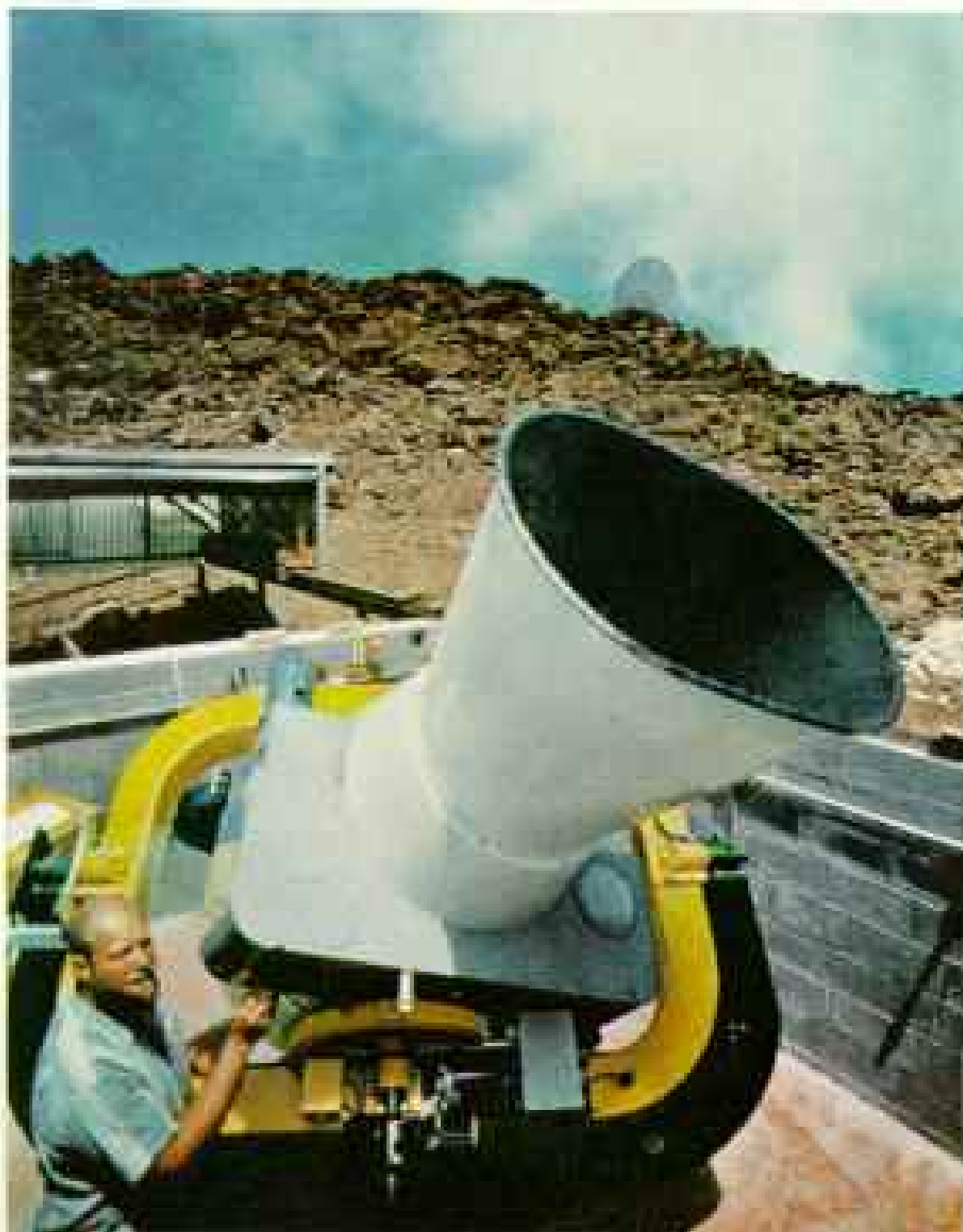
Telescope-with-camera on Maui island daily tracks the satellites man has thrown into space. Twelve such stations belong to Smithsonian's Astrophysical Observatory.
