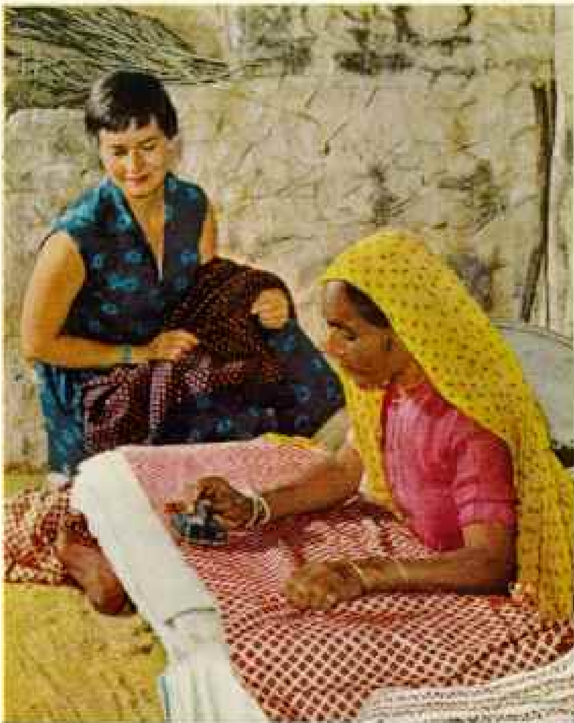
Woman of Sanganer, using an age-old technique, prints designs on cotton. Hand-carved wooden blocks create the pattern.
