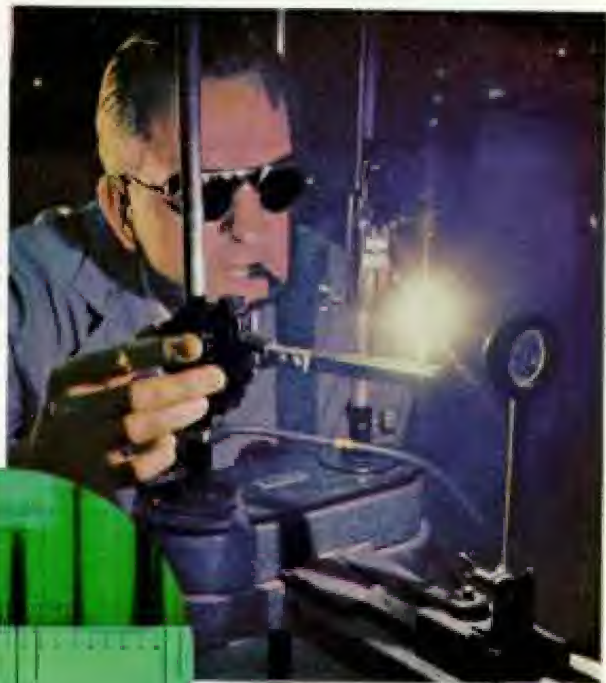
Spectrographic test (above) of particles from wreck shows manganese (Mn, left) from a battery.
