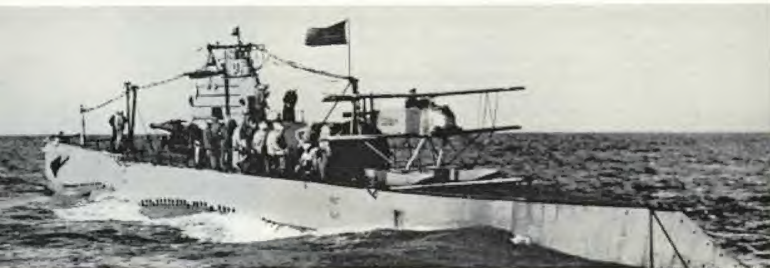
Novel experiment in 1926 saw the submarine S-1 launch a Cox-Klemm NS-1 seaplane off New London, Connecticut. Disassembled, the plane rode in a waterproof tank amidships. Within 12 minutes after the sub surfaced, crewmen could assemble the plane, put it in the water, and watch it take off. To retrieve the plane and submerge again required but 13 minutes.
