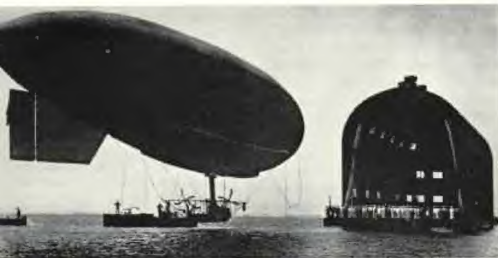
Navy's first airship, the DN-1, approaches its floating hangar on Pensacola Bay, where the twin-propeller gasbag made three successful test flights in April, 1917. Blimps won high praise for their performance during both World Wars. Navy blimp squadrons still operate (page 287).
