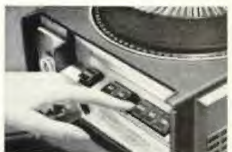
Turn on controls at rear. Keyboard is lighted for easy use in the dark.
