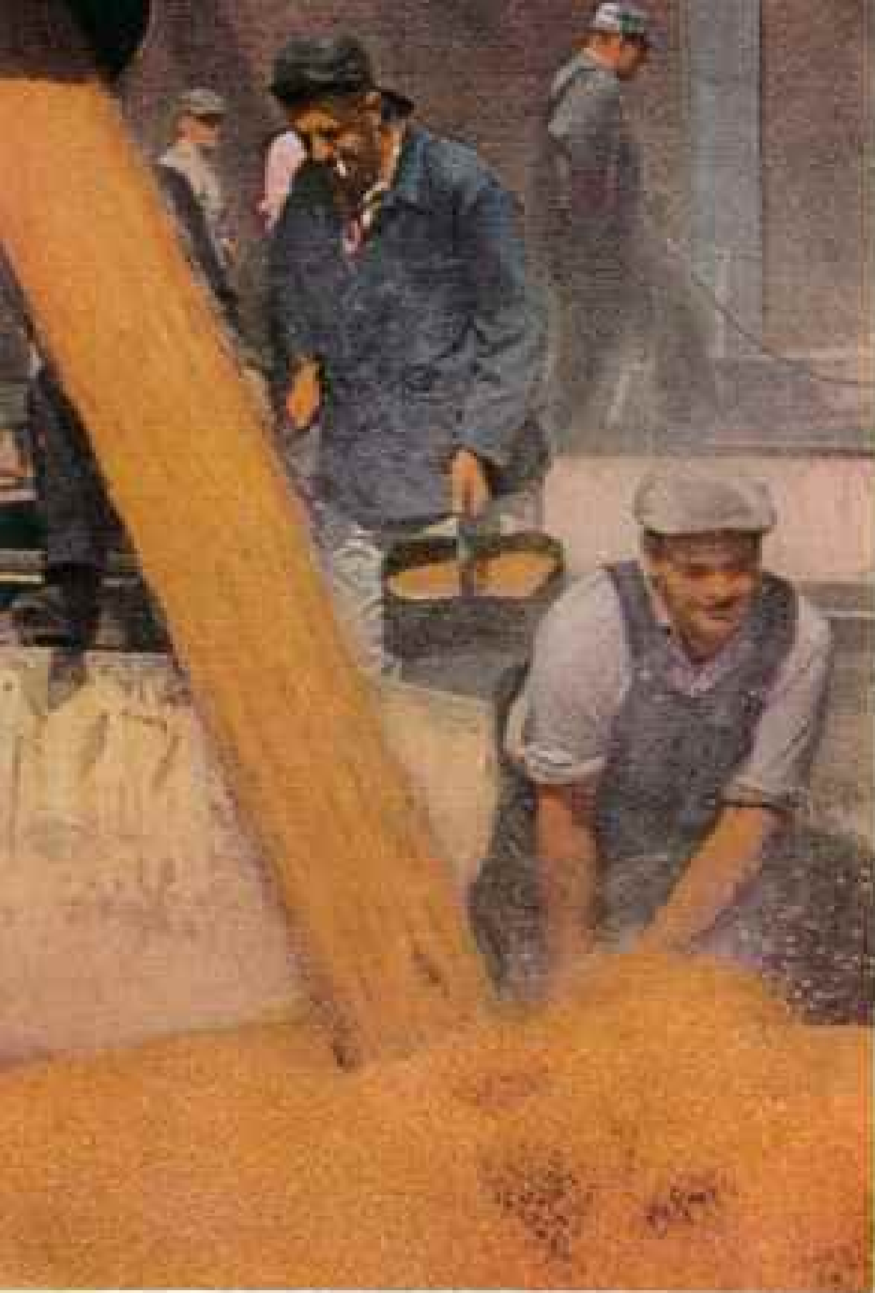
Trimmer distributes wheat pouring from a grain elevator into a ship's hold at Port Arthur, on Lake Superior. Man with a bucket samples the grain for grade and moisture content.
