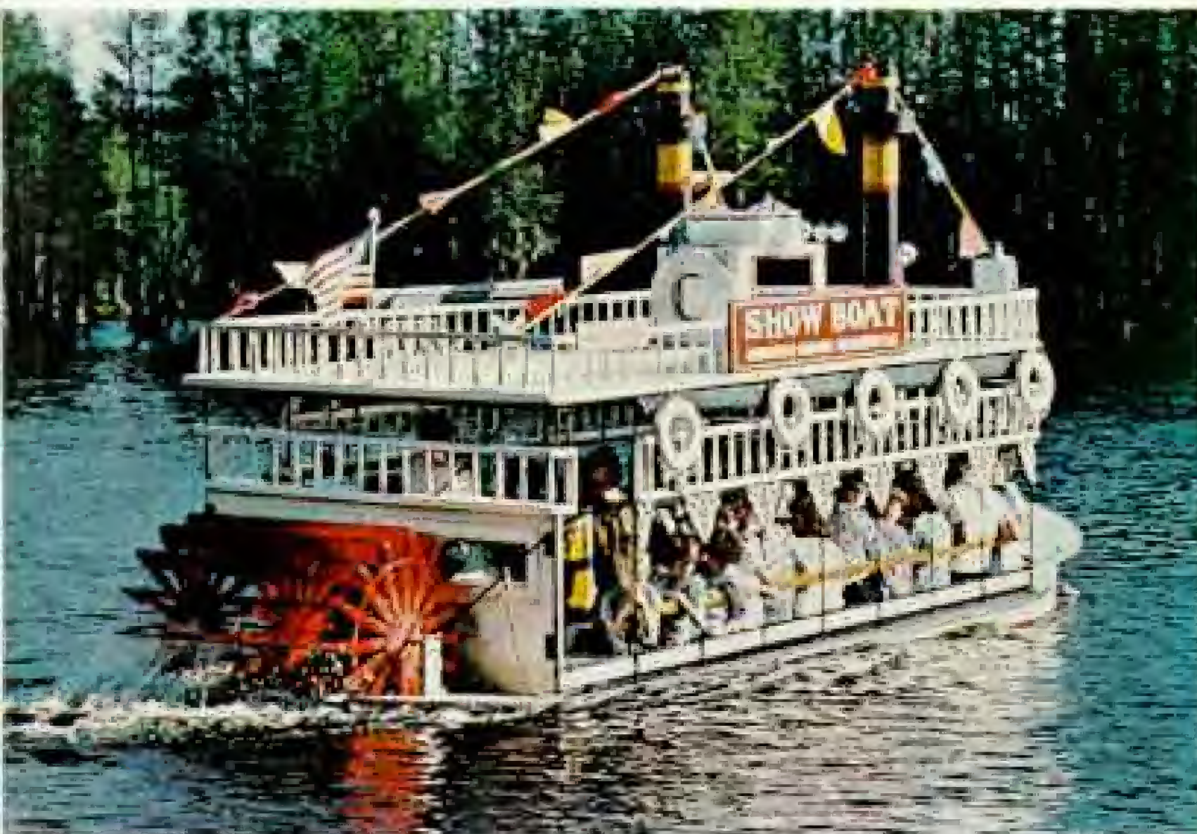
Flags flying, Show Boat carries sightseers around Greenfield Gardens, Wilmington. Motor-driven propeller powers the craft, modeled after old Southern riverboats; its motion turns the paddles. Show Boat seats 32.
