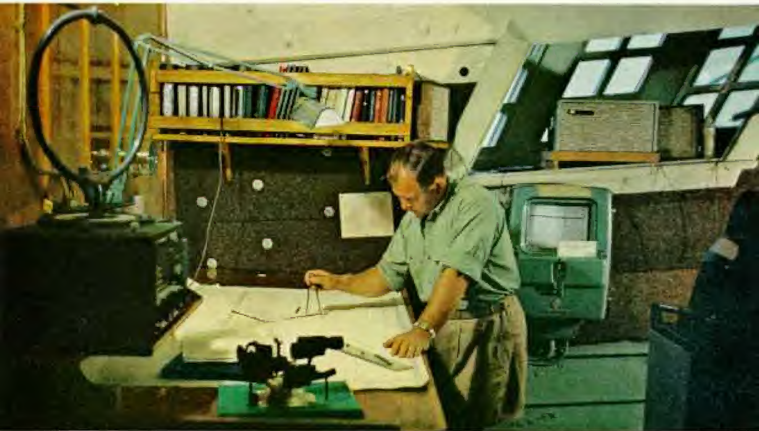
"I have determined the Longitude": Bligh's Jug. Capt. Ellsworth Coggins, master of Bounty , plots his position. Behind him, the depth indicator; at left, the loop of the radio direction finder. Plath sextant stands on the chart table.
