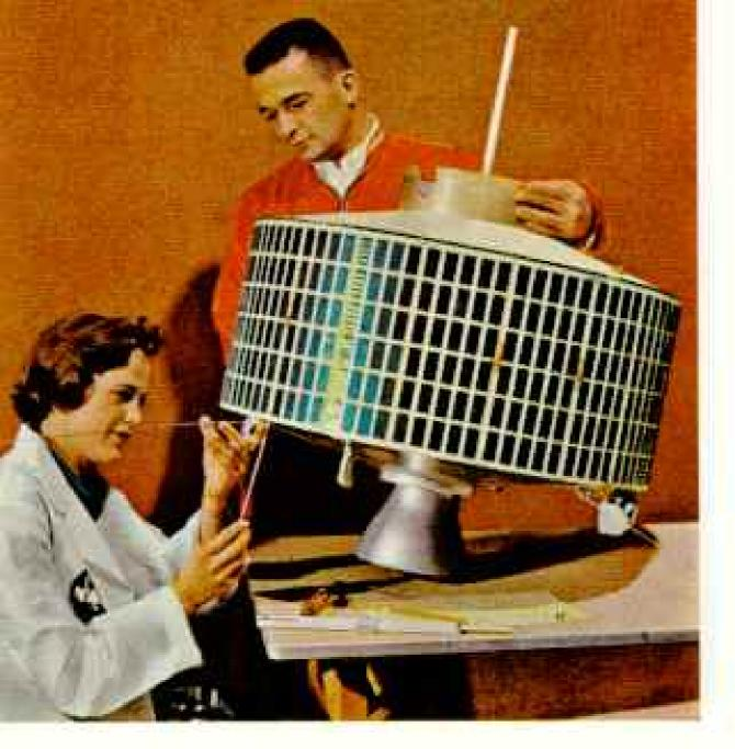
Syncom, Hughes Aircraft's flyweight satellite, will orbit to coincide with the earth's rotation. Here it rests on the nozzle of a small built-in rocket that will give the 60-pound communicator a final kick into synchronous orbit, 22,300 miles high, after a Thor-Delta lifts it from earth. Syncom undergoes tests at the Goddard Space Flight Center, a National Aeronautics and Space Administration facility at Greenbelt. Maryland.
