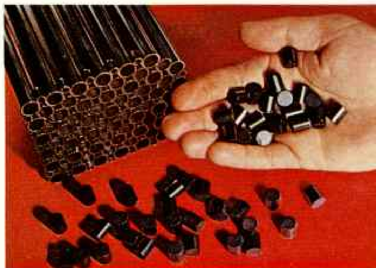
Potent pellets of uranium oxide do the work of coal or oil. Loaded into steel tubes, 815,440 slugs pack enough power to drive the ship 300,000 miles. Until activated, they offer no radiation hazard.
