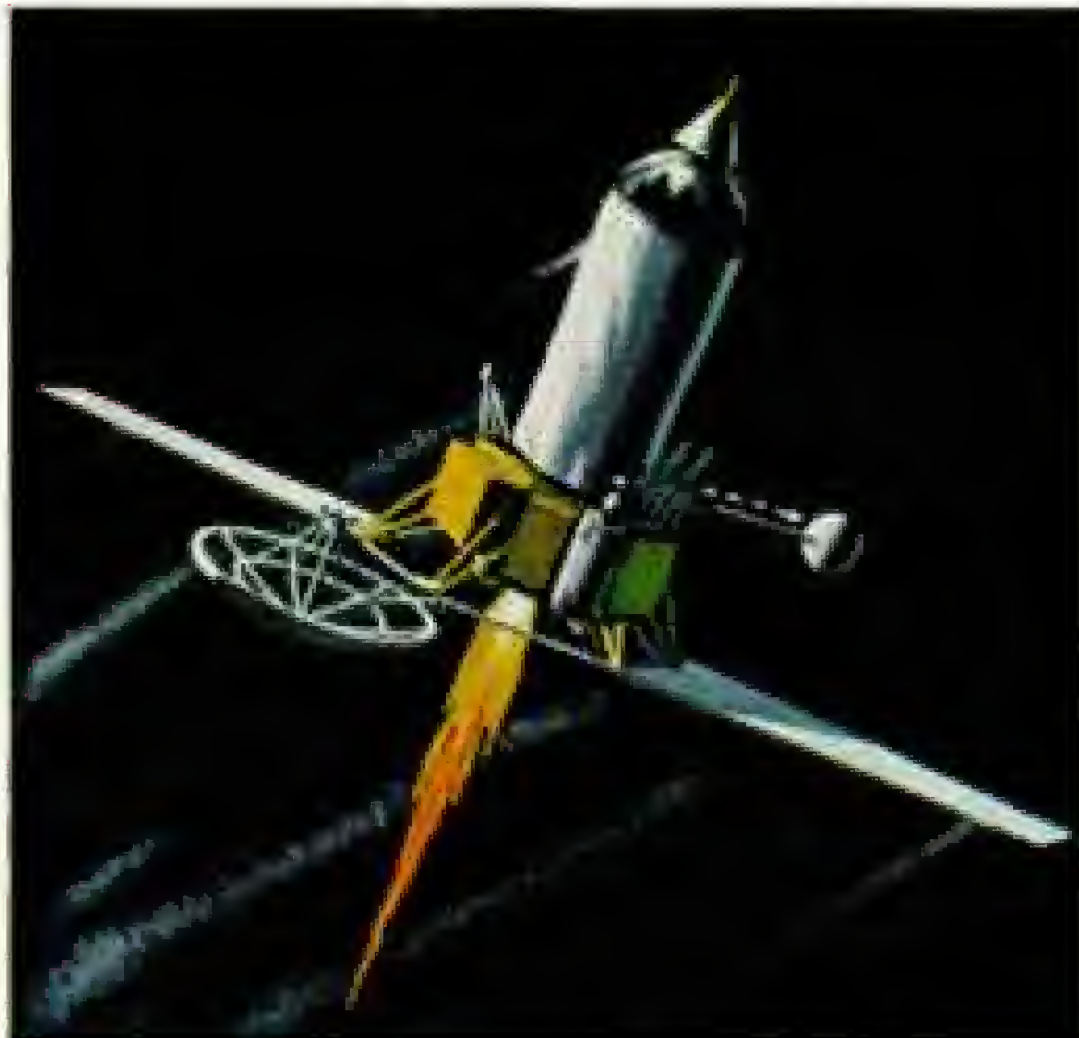
6. Rocket fires on command from ground, placing Ranger on precise course. Then a ball-like gamma-ray counter extends at the end of boom.
