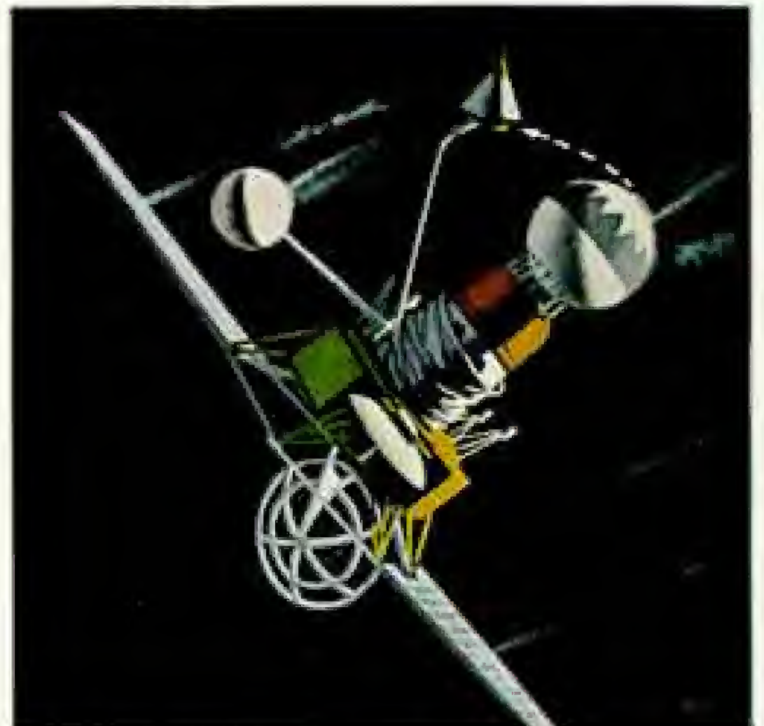
7. Aluminized shroud retracts, exposing the spherical instrument capsule and retrorocket. All-directional antenna (wizard's cap) swings out.
