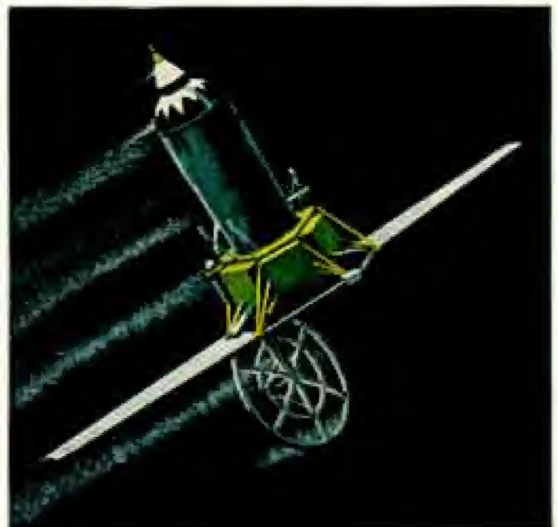
5. Flight attitude is achieved by firing gas jets. Ranger's power-gathering solar panels face the sun; its antenna aims at earth.
