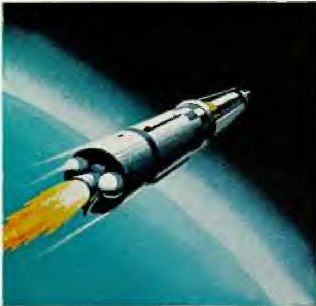
2. Second Agena B firing thrusts Ranger into moon trajectory. Agena's first blast, over the Atlantic, placed the mooncraft in earth orbit.
