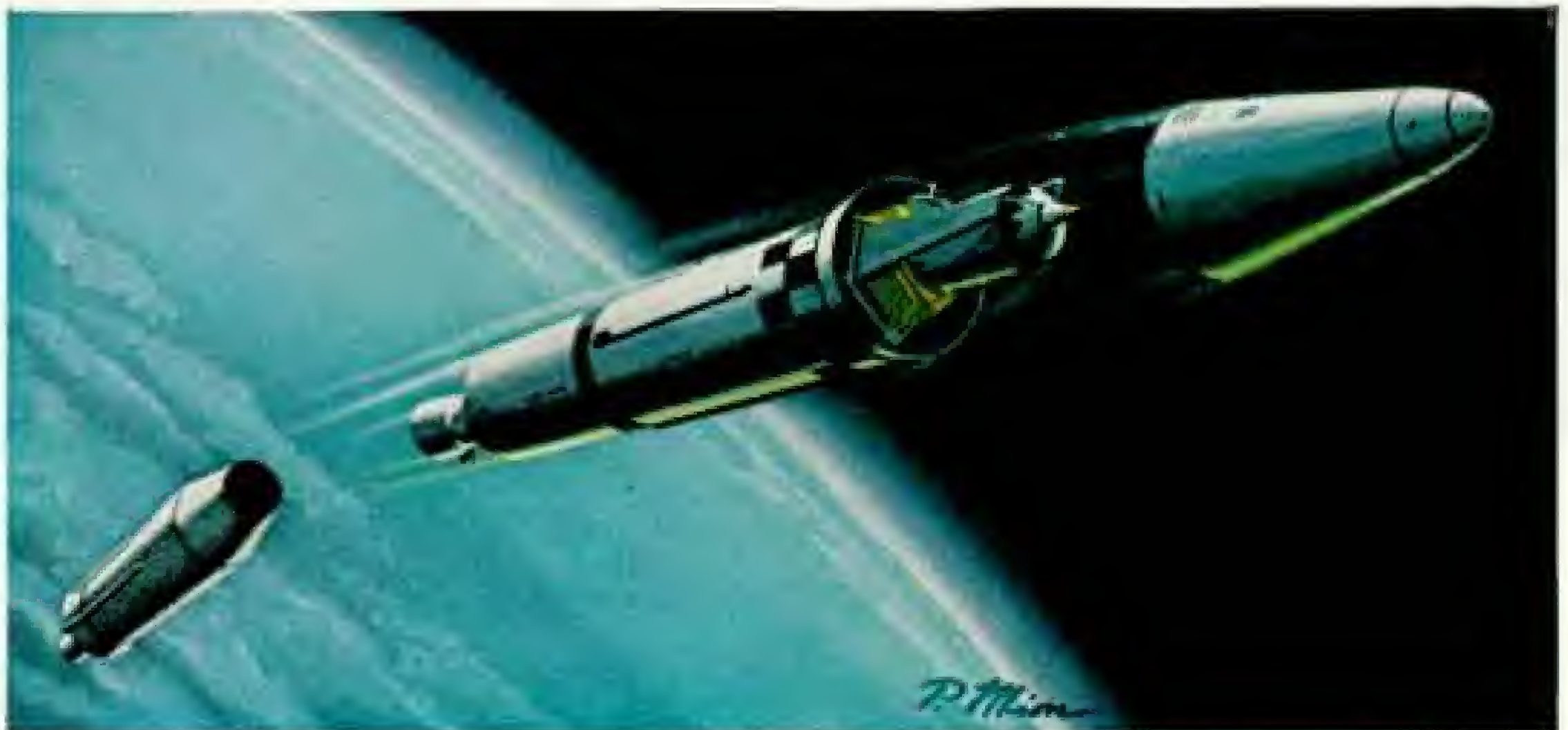
1. One hundred miles above the Atlantic Missile Range, the Agena B-Ranger unit separates from its Atlas booster. Protective nose cone sprang away seconds earlier, exposing Ranger 5. Here and on following pages, artist Pierre Mion shows how this Ranger will function if the venture proves successful.
