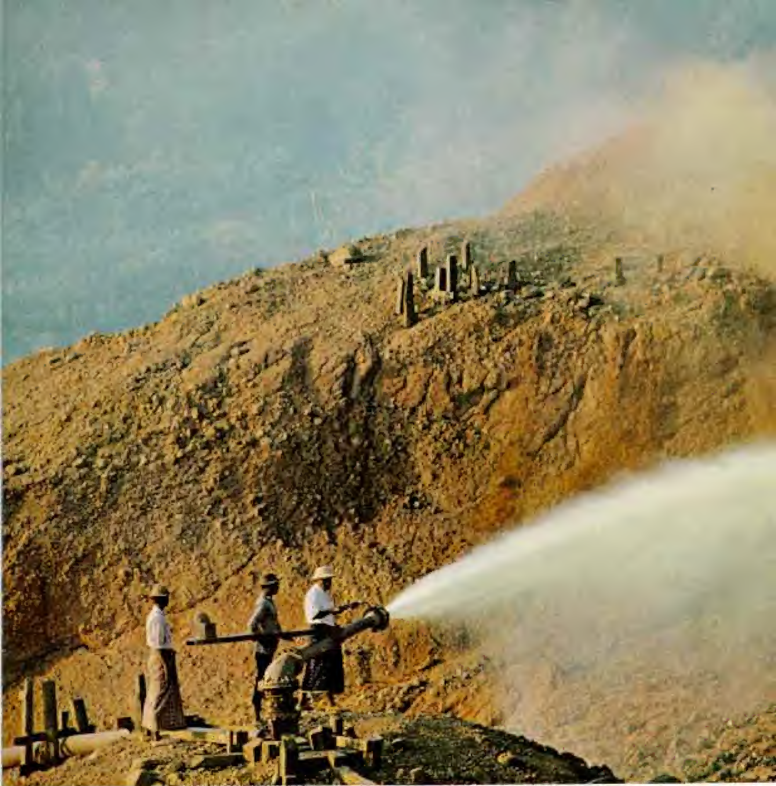
Rushing torrent from a hydraulic jet sluices away a mountainside near Tavoy, on the Tenasserim coast, and redeems tin ore. Torn loose, the red earth flows through catchment boxes that trap fine black granules of cassiterite (tin dioxide).
