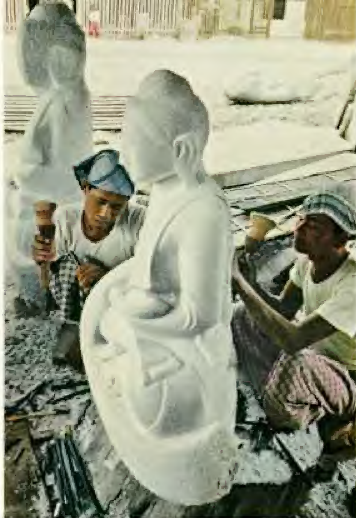
Mandalay artisans on Kyank-sit-tan (Street of the Carvers) shape marble statues of Buddha with mallets and chisels made from old files.
